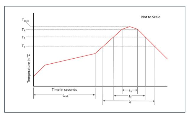
Figure 122: Solder Reflow Profile
