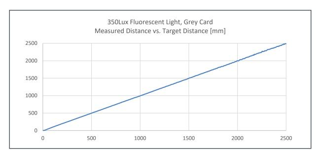
Figure 8: 350 Lux Fluorescent Light, 18% Grey Card and Smudge on Glass
