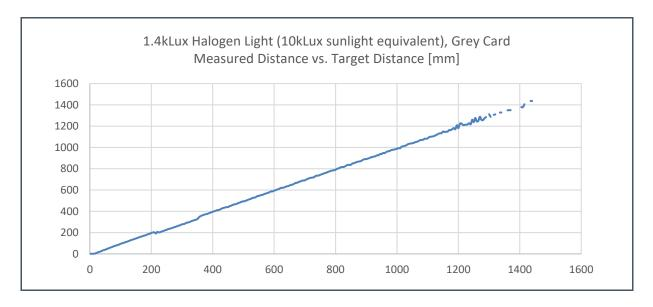
Figure 10: 14k Lux Halogen Light and 18% Grey Card
