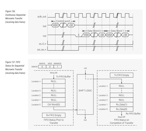
When MDD = 1, this indicates that the DW\_apb\_ssi serial master transmits data to the external serial slave. Immediately after the LSB of the control word is transmitted, the DW\_apb\_ssi master begins transmitting the data frame to the slave peripheral.
