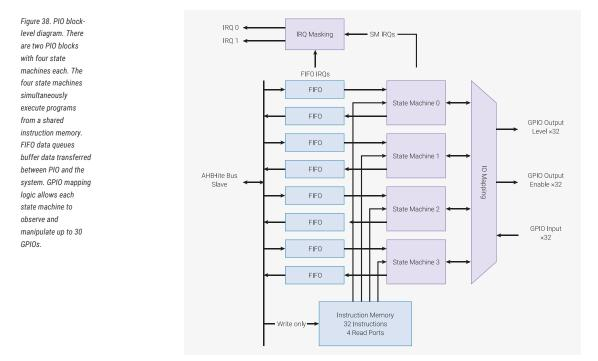
The programmable input/output block (PIO) is a versatile hardware interface. It can support a variety of IO standards, including:
