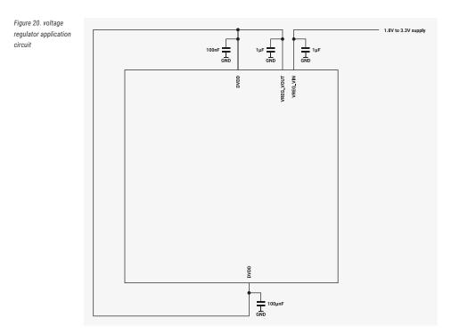
The regulator must have 1µF capacitors placed close to its input (VREG\_VIN) and output (VREG\_VOUT) pins.
