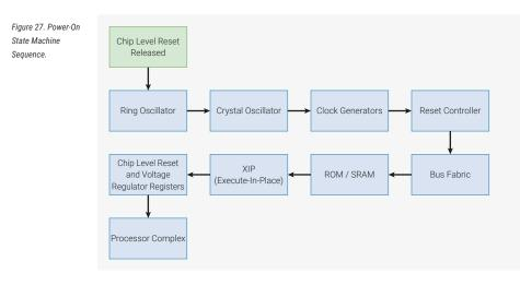
The power-on state machine sequence is as follows:
