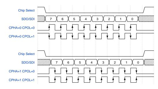
synchronous with a clock (SCK). Two flags. CPOL and CPHA, specify the clock's behaviour. CPOL is the idle state of the clock: 0 for low, 1 for high. The clock pulses a number of times, transferring one bit in each direction per pulse, but always returns to its idle state. CPHA determines on which edge of the clock data is captured: 0 for leading edge, and 1 for trailing edge. The arrows in the figure show the clock edge where data is captured by both the host and device.
