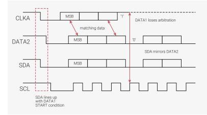
Control of the bus is determined by address or master code and data sent by competing masters, so there is no central master nor any order of priority on the bus.
