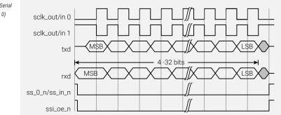
Figure 122. SPI Serial Format (SCPH = 0) The following signals are illustrated in the timing diagrams in this section:
