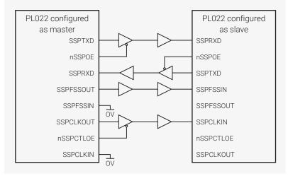
Figure 100 shows how an PrimeCell SSP (PL022), configured as master, interfaces to a Motorola SPI slave. The SPI Slave Select (SS) signal is permanently tied LOW and configures it as a slave. Similar to the above operation, the master can broadcast to the slave through the master PrimeCell SSP SSPTXD line. In response, the slave drives its SPI MISO port onto the SSPRXD line of the master.
