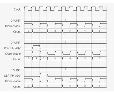
The counter can not count faster than once per cycle, so  $PH_ADV$  requires  $DIV_INT > 1$  or  $DIV_FRAC > 0$ . Likewise, the counter will not start to count backward if  $PH_RET$  is asserted when the clock enable is permanently low.
