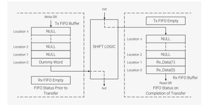
For eeprom\_read transfers (transfer mode field [9:8] of the Control Register 0 = 11b), opcode and/or EEPROM address are written into the transmit FIFO. During transmission of these control frames, received data is not captured by the DW\_apb\_ssi master. After the control frames have been transmitted, receive data from the EEPROM is stored in the receive FIFO.
