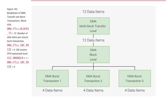
If the DW\_apb\_ssi makes a transmit request to this channel, four data items are written to the DW\_apb\_ssi transmit FIFO. Similarly, if the DW\_apb\_ssi makes a receive request to this channel, four data items are read from the DW\_apb\_ssi receive FIFO. Three separate requests must be made to this DMA channel before all 12 data items are written or read.
