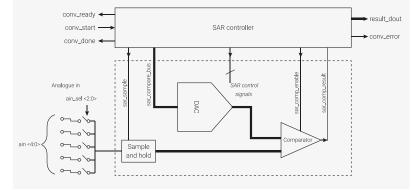
The ADC requires a 48MHz clock (  $clk_adc$  ), which could come from the USB PLL. Capturing a sample takes 96 clock cycles (96 x 1 / 48MHz) = 2 µs per sample (500kS/s). The clock must be set up correctly before enabling the ADC.
