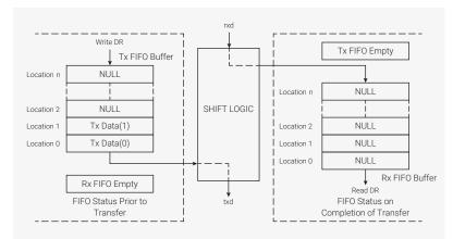
For receive only transfers (transfer mode field (9:8) of the Control Register 0 = 10b), data transmitted from the DW\_apb\_ssi to the external serial device is invalid, so a single dummy word is written into the transmit FIFO to begin the serial transfer. The txd output from the DW\_apb\_ssi is held at a constant logic level for the duration of the serial transfer. Data received
