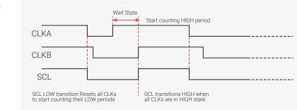
Figure 82. Multi-Master Clock Synchronization
