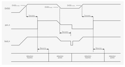
Once the chip is out of reset, detection can be disabled under software control. This also saves a small amount of power. If detection is subsequently re-enabled, there will be another short delay, the *brown-out detection enable delay* ( $t_{BOD.ENABLE}$ ), before it becomes active again. This is shown in Figure 25.
