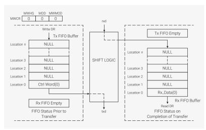
Continuous transfers for the Microwire protocol can be sequential or nonsequential, and are controlled by the MWMOD bit field (bit 0) in the MWCR register.
