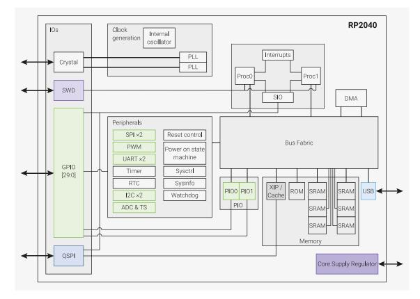
Code may be executed directly from external memory through a dedicated SPI, DSPI or QSPI interface. A small cache improves performance for typical applications.
