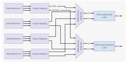
Each state machine may assert an OUT/SET and a side-set through its pin mapping hardware on each cycle. This generates 32 bits of write data and write mask for the GPIO output level and output enable registers, from each state machine.
