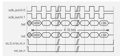
Continuous data frames are transferred in the same way as single frames, with the MSB of the next frame following directly after the LSB of the current frame. The slave select signal is held active for the duration of the transfer.
