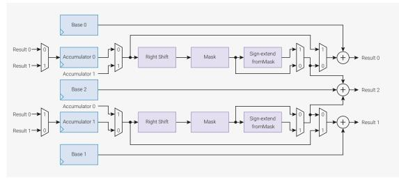
The processor can write or read any interpolator register in one cycle, and the results are ready on the next cycle. The processor can also perform an addition on one of the two accumulators ACCUM0 or ACCUM1 by writing to the corresponding ACCUM\_ADD register.
