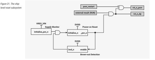
The chip level reset subsystem is shown in Figure 21, and more information is available in the following sections.
