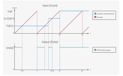
The behaviour becomes even more perplexing if the TOP register is also modified. It would be difficult for software to write to CC or TOP with the correct timing. To solve this, each slice has two copies of the CC and TOP registers: one copy which software can modify, and another, internal copy which is updated from the first register at the instant the counter wraps. Software can modify its copy of the register at will, but the changes are not captured by the PWM output until the next wrap.
