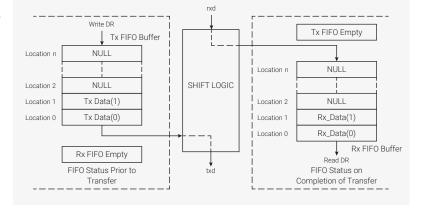
For transmit only transfers (transfer mode field (9:8) of the Control Register 0 = 01b), data transmitted from the DW\_apb\_ssi to the external serial device is written into the transmit FIFO. As the data received from the external serial device is deemed invalid, it is not stored in the DW\_apb\_ssi receive FIFO.
