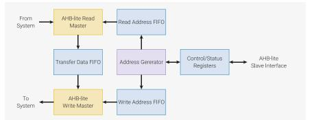
The DMA can perform one read access and one write access, up to 32 bits in size, every clock cycle. There are 12 independent channels, each which supervise a sequence of bus transfers, usually in one of the following scenarios:
