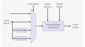
By default, each slice's counter is free-running, and will count continuously whenever the slice is enabled. There are three other options available:
