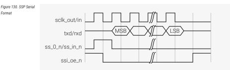
Continuous data frames are transferred in the same way as single data frames. The frame indicator is asserted for one clock period during the same cycle as the LSB from the current transfer, indicating that another data frame follows.
