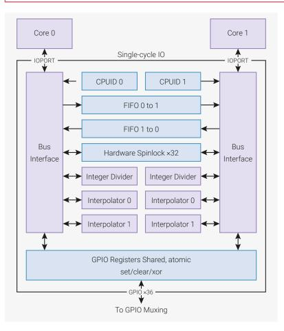
All IOPORT reads and writes (and therefore all SIO accesses) take place in exactly one cycle, unlike the main AHB-Lite system bus, where the Cortex-M0+ requires two cycles for a load or store, and may have to wait longer due to contention from other system bus masters. This is vital for interfaces such as GPIO, which have tight timing requirements.
