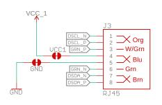
Cut traces on VCC1 and GND jumpers to disconnect VCC1 and GND from cable.
