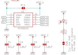
VCC: I2C-bus side power supply (2.3V-5.5V) VCC1: Differential side power supply (3.0V-5.5V)
