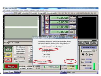
Step 2: Power on the control box and switch the power switch to ON. At this time, the emergency reset button "Reset" in the lower left corner of the computer control interface is flashing.
