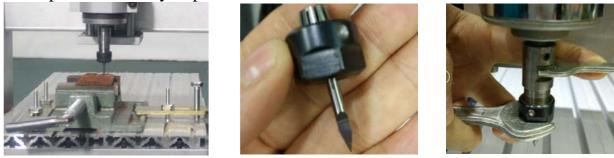
Step 2: Clamp the tool onto the spindle motor. When clamping the tool, it is necessary to pay attention to the specifications of the clamping tool. It must be the same as the programming time. The tool should be locked with the spindle wrench. After the tool is clamped, it must be
