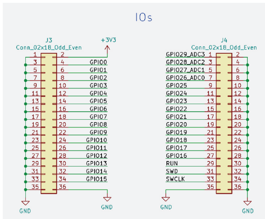
Figure 10. Schematic section showing the 2.54mm IO headers
