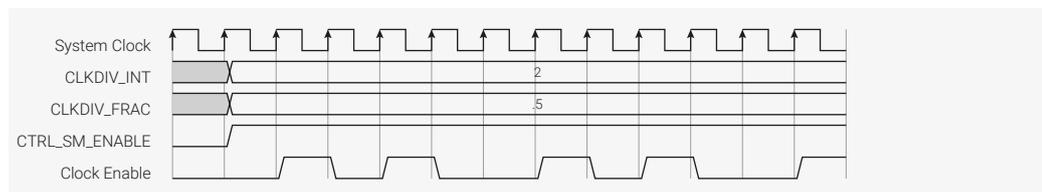
For small  $n$ , the jitter introduced by a fractional divider may be unacceptable. However, for larger values, this effect is much less apparent.
