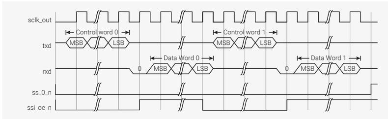
The only modification needed to perform a continuous nonsequential transfer is to write more control words into the transmit FIFO buffer; this is illustrated in Figure 135. In this example, two data words are read from the external serial-slave device.
