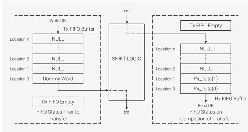
For eeprom\_read transfers (transfer mode field [9:8] of the Control Register 0 = 11b), opcode and/or EEPROM address are written into the transmit FIFO. During transmission of these control frames, received data is not captured by the DW\_apb\_ssi master. After the control frames have been transmitted, receive data from the EEPROM is stored in the receive FIFO.
