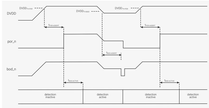
Once the chip is out of reset, detection can be disabled under software control. This also saves a small amount of power. If detection is subsequently re-enabled, there will be another short delay, the *brown-out detection enable delay* ( $t_{BOD.ENABLE}$ ), before it becomes active again. This is shown in Figure 25.
