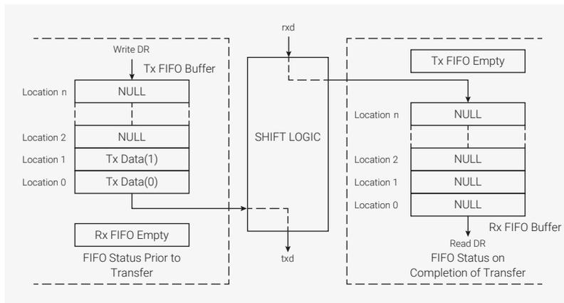
For receive only transfers (transfer mode field (9:8) of the Control Register 0 = 10b), data transmitted from the DW\_apb\_ssi to the external serial device is invalid, so a single dummy word is written into the transmit FIFO to begin the serial transfer. The txd output from the DW\_apb\_ssi is held at a constant logic level for the duration of the serial transfer. Data received
