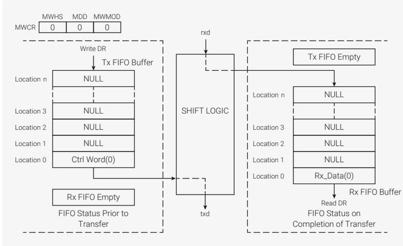
Continuous transfers for the Microwire protocol can be sequential or nonsequential, and are controlled by the MWMOD bit field (bit 0) in the MWCR register.
