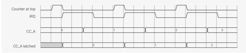
There is no limitation on what values can be written to **CC** or **TOP**, or when they are written. In normal PWM mode (**CSR\_PH\_CORRECT** is 0) the latched copies are updated when the counter wraps to 0, which occurs once every **TOP** + 1 cycles. In phase-correct mode (**CSR\_PH\_CORRECT** is 1), the latched copies are updated on the 0 to 0 count transition, i.e. the point where the counter stops counting downward and begins to count upward again.
