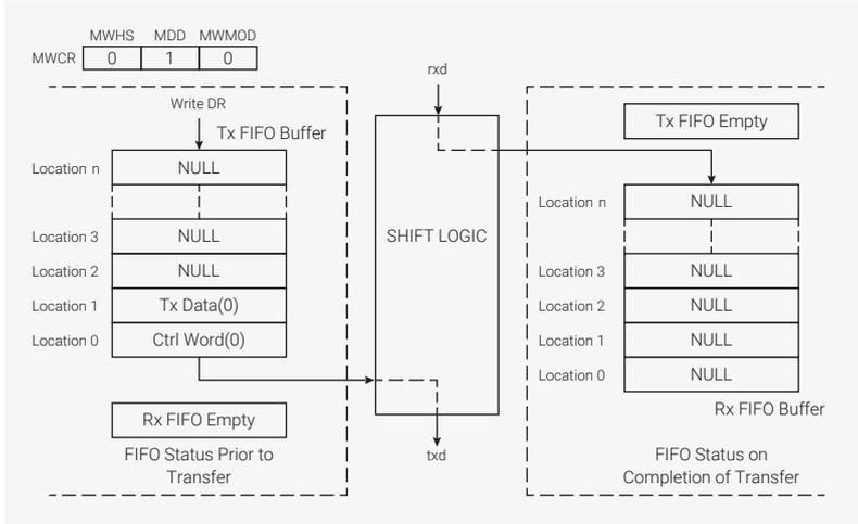
Continuous transfers occur as shown in Figure 140, with the control word for the next transfer following immediately after the LSB of the current data word.
