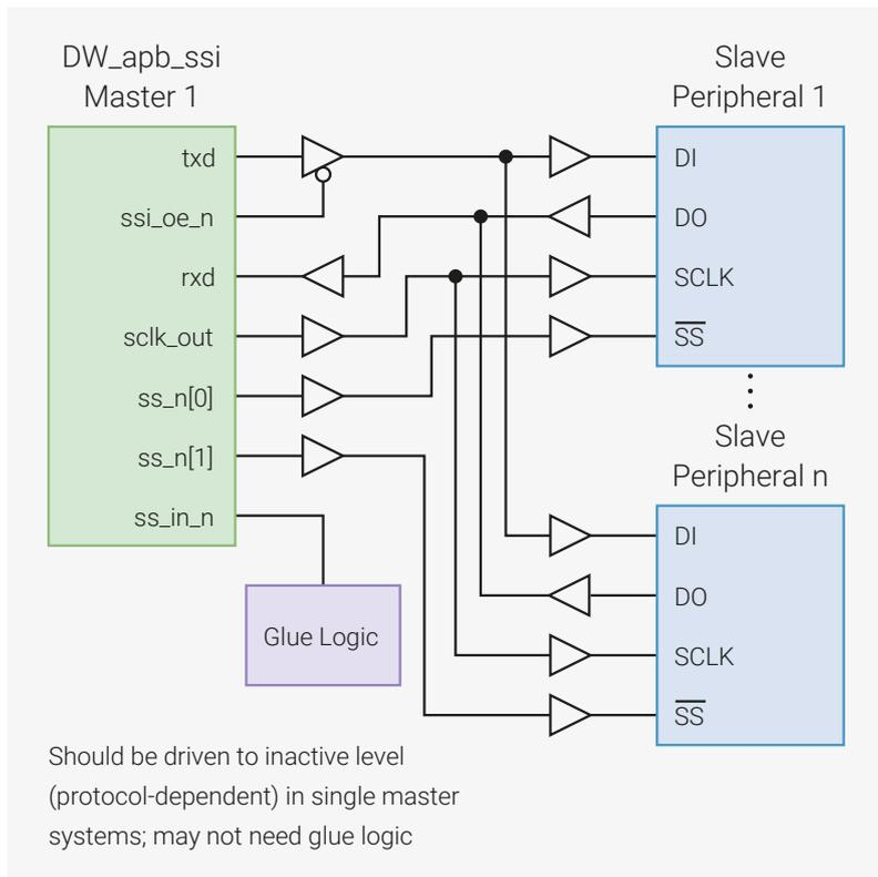
The serial bit-rate clock, generated and controlled by the DW\_apb\_ssi, is driven out on the sclk\_out line. When the DW\_apb\_ssi is disabled (SSL\_EN = 0), no serial transfers can occur and sclk\_out is held in “inactive” state, as defined by the serial protocol under which it operates.
