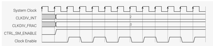
Fractional division will maintain a steady state division rate of  $n + f / 256$ , where  $n$  and  $f$  are the integer and fractional fields of this state machine's **CLKDIV** register. It does this by selectively extending some division periods from  $n$  cycles to  $n + 1$ .
