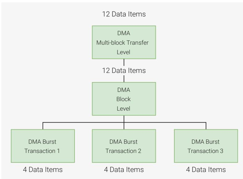
If the DW\_apb\_ssi makes a transmit request to this channel, four data items are written to the DW\_apb\_ssi transmit FIFO. Similarly, if the DW\_apb\_ssi makes a receive request to this channel, four data items are read from the DW\_apb\_ssi receive FIFO. Three separate requests must be made to this DMA channel before all 12 data items are written or read.
