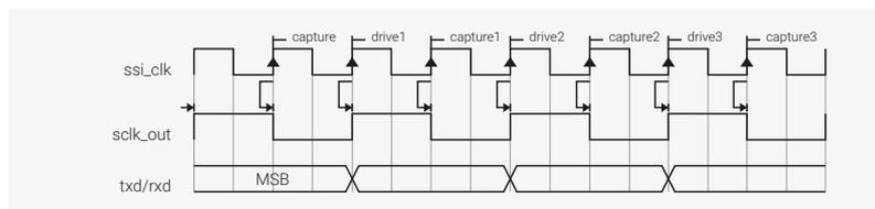
The sclk\_out line toggles only when an active transfer is in progress. At all other times it is held in an inactive state, as defined by the serial protocol under which it operates.
