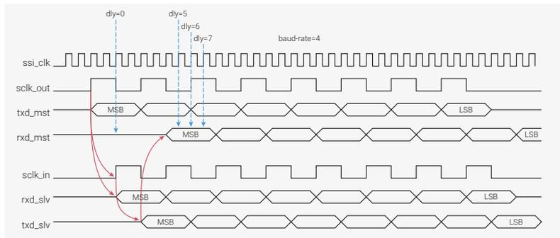
The Slave uses the sclk\_out signal from the master as a strobe in order to drive rxd signal data onto the serial bus. Routing and sampling delays on the sclk\_out signal by the slave device can mean that the rxd bit has not stabilized to the correct value before the master samples the rxd signal. Figure 119 shows an example of how a routing delay on the rxd signal can result in an incorrect rxd value at the default time when the master samples the port.
