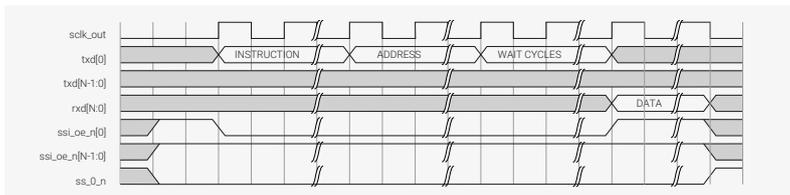
**Case B: Instruction transmitted in standard and address transmitted in dual SPI format**
