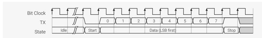
We can recover the data by waiting for the start bit, sampling 8 times with the correct timing, and pushing the result to the RX FIFO. Below is possibly the shortest program which can do this:
