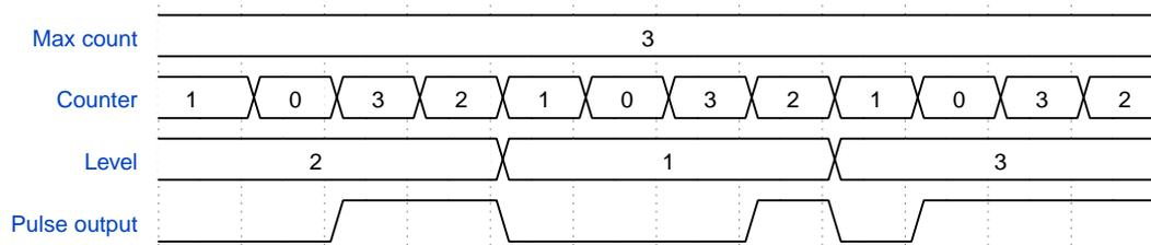
This program repeatedly counts down to 0 with the Y register, whilst comparing the Y count to a pulse width held in the X register. The output is asserted low before counting begins, and asserted high when the value in Y reaches X. Once Y reaches 0, the process repeats, and the output is once more driven low. The fraction of time that the output is high is therefore proportional to the pulse width stored in X.
