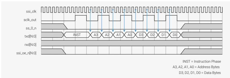
Figure 160. Transmit Data With DDR\_DRIVE\_EDGE = 2
