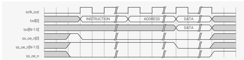
**Case B: Instruction transmitted in standard and address transmitted in Enhanced SPI format**
