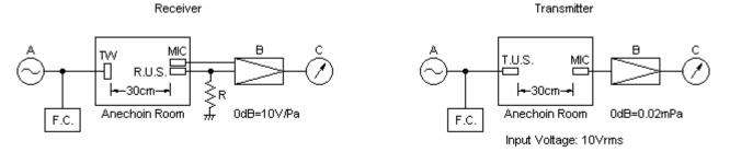
A: Oscillator B: Amplifier C: Voltmeter R: 3.9K MIC: Microphone TW: Tweeter R:U.S.: Receiver Ultrasonic Sensor T:U.S.: Transmitter Ultrasonic Sensor F.C.: Frequency Counter
