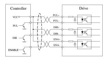
Figure 3: Connections to open-collector signal (common-anode)
