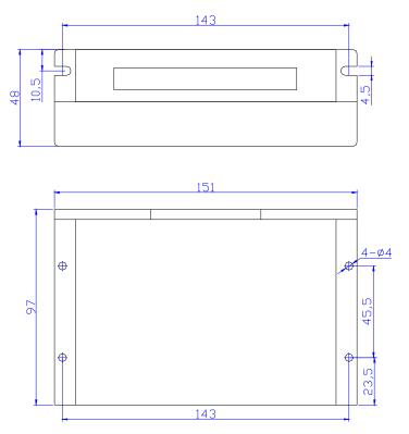
Figure 1: Mechanical specifications \*Recommend use side mounting for better heat dissipation
