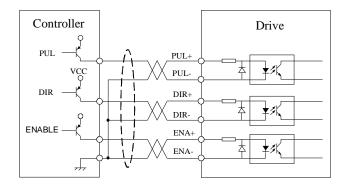
Figure 4: Connection to PNP signal (common-cathode)
