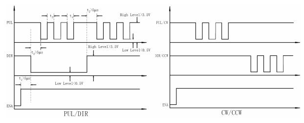
Figure 11: Sequence chart of control signals
