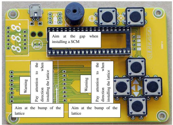
2. Weld the lattice module. There is a small block under the silk-screen on the PCB as well as a bump at the lattice edge, correspond the block with the bump.
