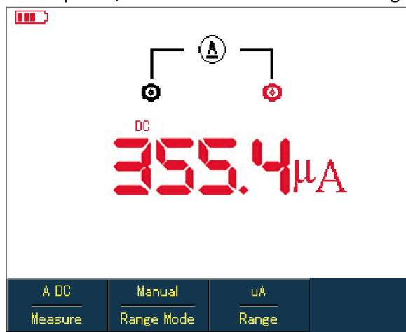
Figure 5-7 Measuring DC Current lower than 4Ma
