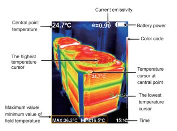
Color code: used to mark the color corresponding to the relative temperature from low to high in the field of version.
