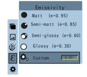
As shown in the figure, press "  $\oplus$  / MENU" key to enter the main menu and select "  $\pounds$  "(emissivity) option and press "  $\blacktriangleright$  " key to enter the emissivity list.
