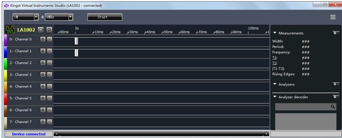
From this figure, we can see the coordinate values of the time axis are too large, and the effective waveform is within a very short period. You can click the left button of the mouse to zoom out the waveform; while the right button would zoom it in. And you can get these done with the mouse wheel too. After the waveform is zoomed up, you could see:
