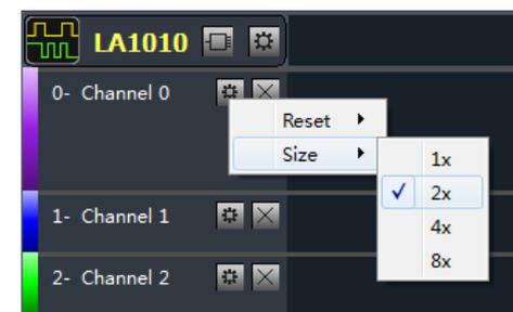
If you press “reset” in this menu, you could reset the channels to default state, for example default size, name, etc.
