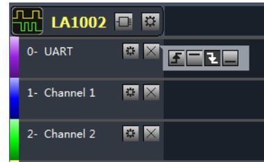
After the trigger is set and the button “start” is pressed again, if the trigger condition (falling edge) we have set have not appeared on channel 0, the logic analyzer would stay in wait state until the falling edge arrives. Then the device will sample and save the data, and upload the data to the computer for displaying and analyzing when the process is complete.
