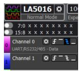
Indicates "rising edge trigger". Indicates "high level trigger".
