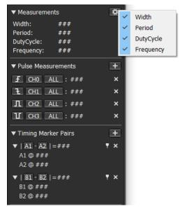
After some items have been selected, move the mouse inside the waveform window, the measurement results of where the mouse stays would display in the measurement window.
