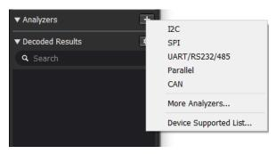
Click the "More Analyzers", and all the supported analyzers will be listed, as shown in the figure below.
