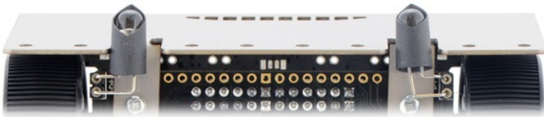
IR LEDs with heat shrink shielding.
