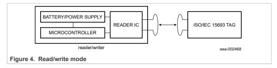
A typical system using the SLRC610 is using a microcontroller to implement the higher levels of the contactless communication protocol and a power supply (battery or external supply).
