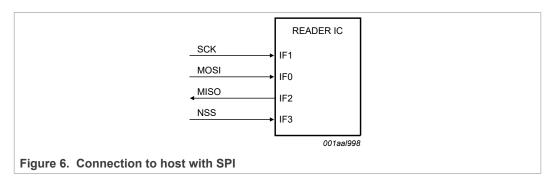
The SLRC610 acts as a slave during the SPI communication. The SPI clock SCK has to be generated by the master. Data communication from the master to the slave uses the Line MOSI. Line MISO is used to send data back from the SLRC610 to the master.
