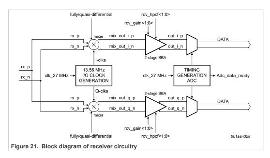
The receiver can also be operated in a single ended mode. In this case the Rcv\_RX\_single bit has to be set. In the single ended mode, the two receiver pins RXP and RXN need to be connected together and will provide a single ended signal to the receiver circuitry.
