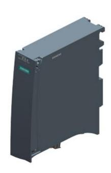
SIPLUS ET 200MP IM 155-5 PN ST -40°C to +70°C with conformal coating based on 6ES7155-5AA01-0AB0 . PROFINET IO device Interface module IM 155-5 PN ST for ET 200MP "electronic modules; up to 12 IO" modules without PS up to 30 IO modules with additional PS "Integrated 2-port switch; RJ45" "shared device; MRP IRT >=0.25" "ms; Isochronous mode FW update;" "I&M0...3; FSU with 500 ms"
