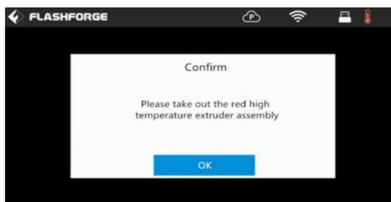
**Guidur IIS is updated, the extruder support 300 degree. The high temp extruder mode will be set before leaving factory.**
