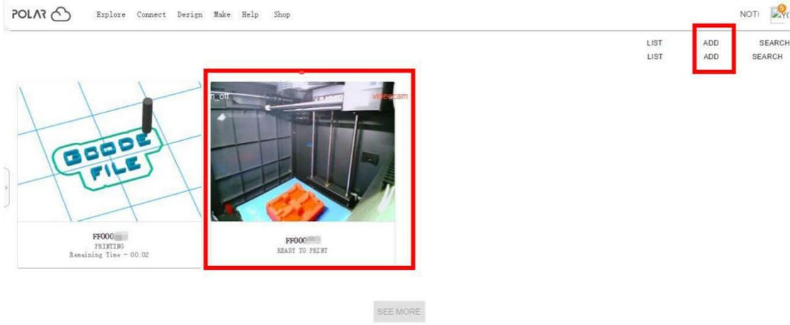
5) By using Polar3D Cloud platform, you can create G-CODE printing job by uploading your own sliced print files. Print files can be transferred to corresponding printer and printing will be started automatically. You can also adjust the extruder temperature, or explore other cloud functions.
