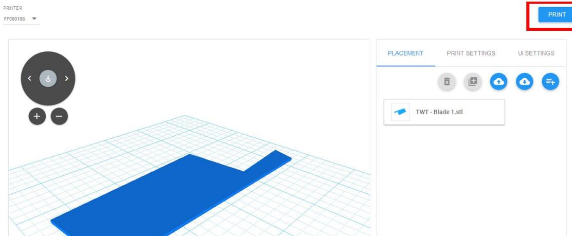
Tap **【START】** button, the printer starts downloading printing file automatically, after downloading completed, you can interactively operate the printer on your computer, including Change Filament, Pause, Stop etc.
