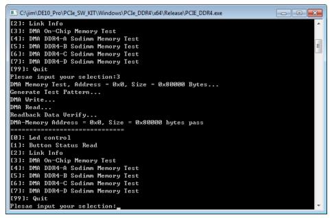
Figure 7-18 Screenshot of On-Chip Memory DMA Test Result
