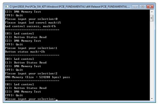
Figure 7-14 Screenshot of DMA Memory Test Result
