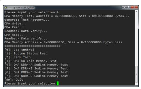
Figure 8-13 Screenshot of DDR4-A SOSIMM Memory DAM Test Result
