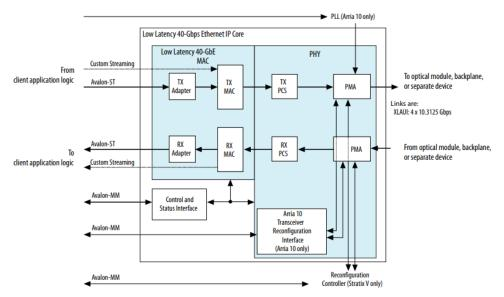
Figure 9-10 Block diagram of 40GbE demo
