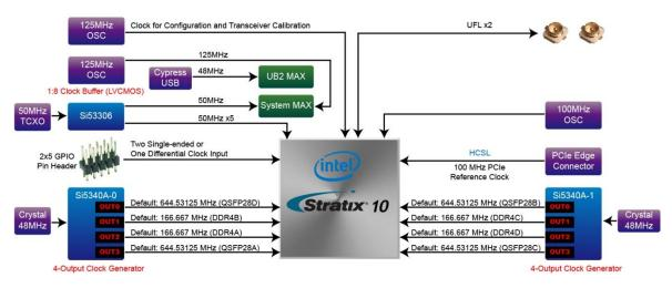
Figure 5-1 The clock tree of the DE10-Pro
