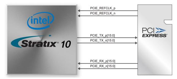
Figure 2-16 PCI Express pin connection
