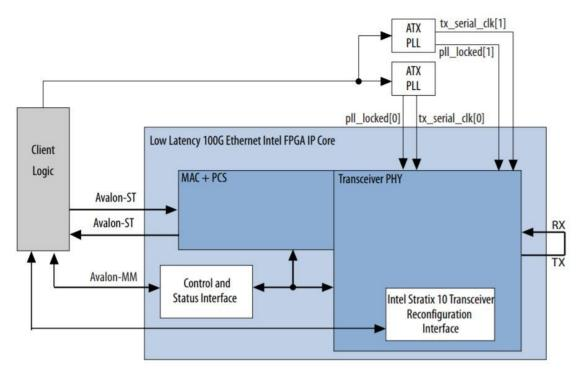
Figure 9-6 Block diagram of 100GbE demo
