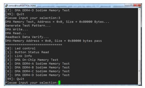
Figure 8-12 Screenshot of On-Chip Memory DMA Test Result
