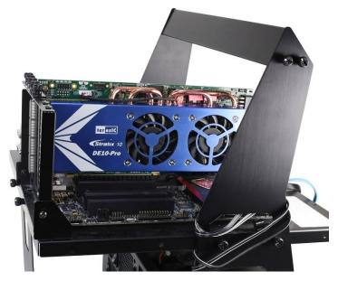
Figure 8-4 FPGA board installation on PC
