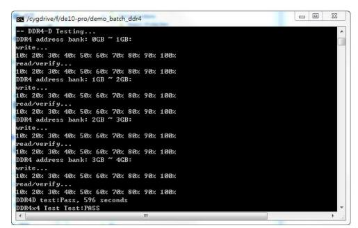
Figure 6-5 Progress and Result Information for the DDR4D Demonstration
