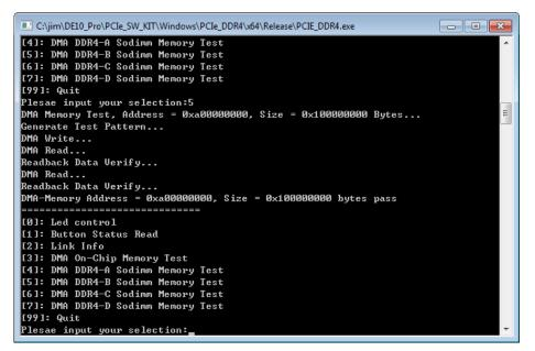
Figure 7-20 Screenshot of the DDR4-B SOSIMM Memory DMA Test Result
