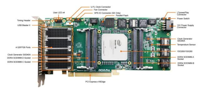
Figure 2-1 FPGA Board (Top)
