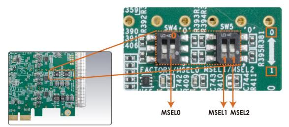
Figure 2-3 Position of slide switches SW4 and SW5 for Configuration Mode
