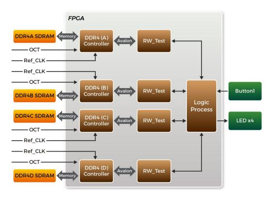
Figure 6-1 Block diagram of DDR4 SDRAM (4G) x4 demonstration
