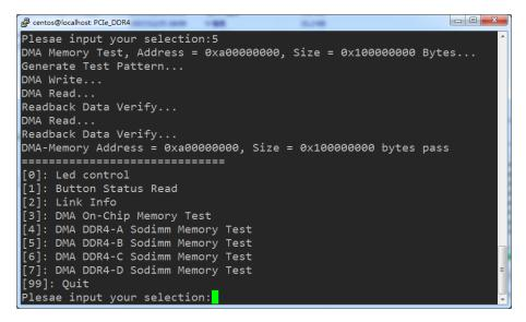
Figure 8-14 Screenshot of DDR4-B SOSIMM Memory DAM Test Result
