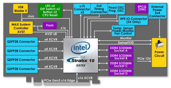
Figure 1-1 Block diagram of the DE10-Pro board
