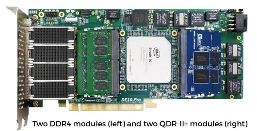
Figure 2-14 Two memory module insertion examples
