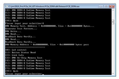
Figure 7-19 Screenshot of the DDR4-A SOSIMM Memory DMA Test Result
