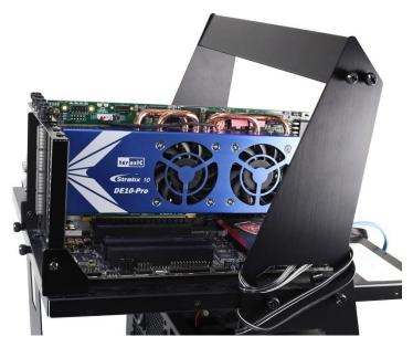
Figure 7-9 FPGA board installation on PC
