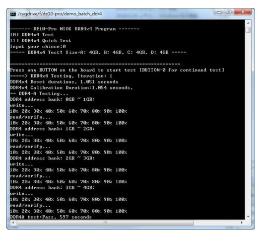
Figure 6-3 Progress and Result Information for the DDR4A Test
