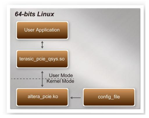
Figure 8-2 PCI Express Software Stack
