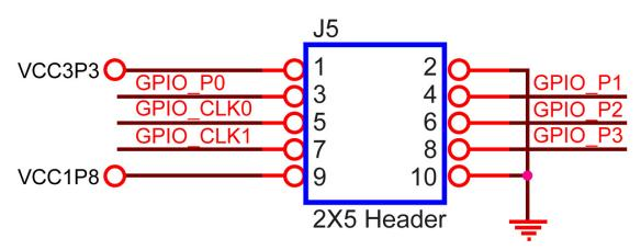
Figure 2-7 Pin-out of 2x5 expansion header J5
