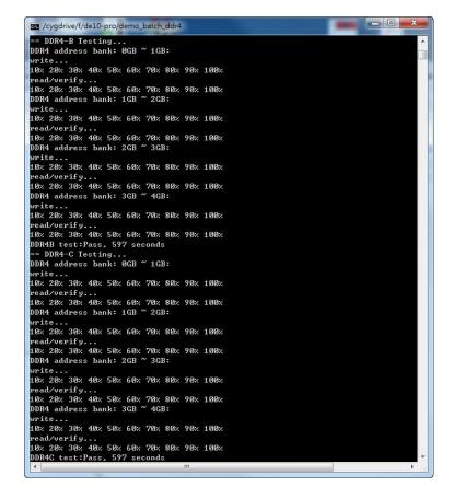
Figure 6-4 Progress and Result Information for the DDR4B and DDR4C Test
