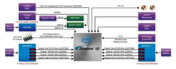
Figure 2-11 Clock circuit of the FPGA Board
