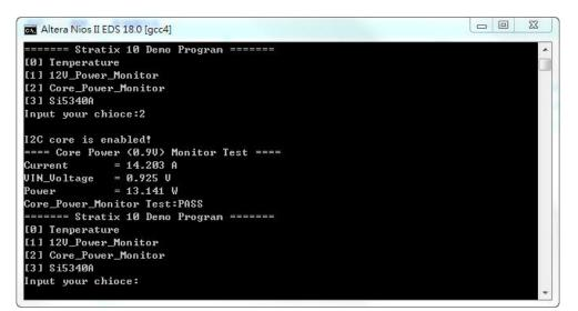
Figure 5-12 Core power monitor Demo
