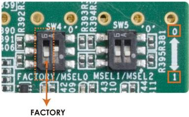
Figure 4-2 Configuration Image Selection
