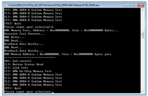
Figure 7-21 Screenshot of the DDR4-C SOSIMM Memory DMA Test Result
