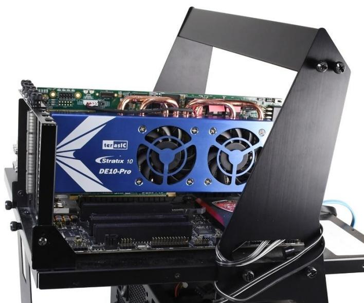
Figure 8-4 FPGA board installation on PC
