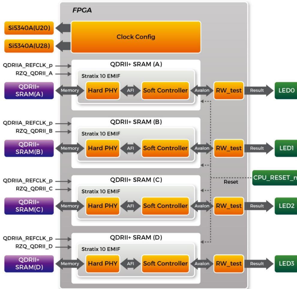
Figure 6-7 Function Block Diagram of the QDRII+ SRAM x4 Demonstration
