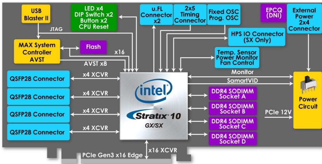
Figure 1-1 Block diagram of the DE10-Pro board
