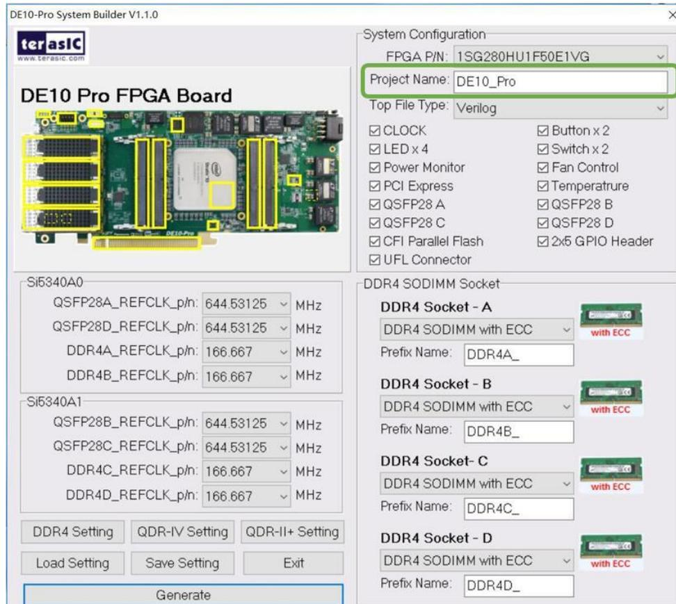
Figure 3-4 Project Name in the System Builder window
