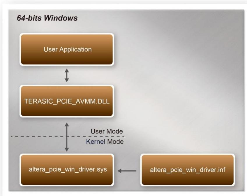
**Figure 7-2 PCI Express Software Stack**
