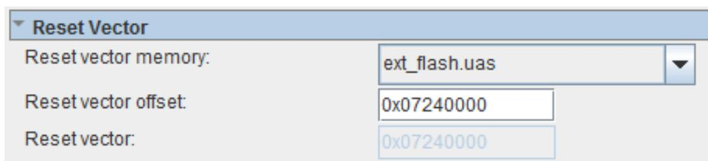
Figure 4-9 User Software Reset Vector Settings for NIOS II Processor
