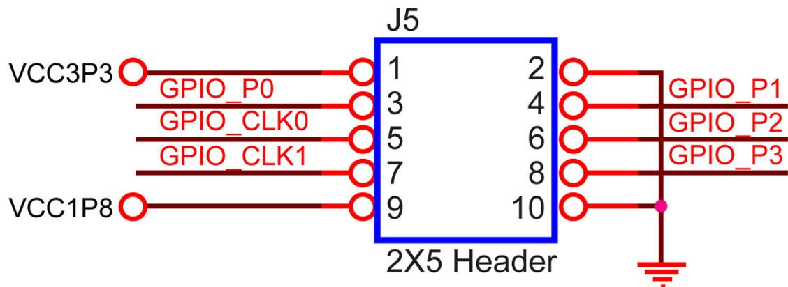
**Figure 2-7** Pin-out of 2x5 expansion header J5
