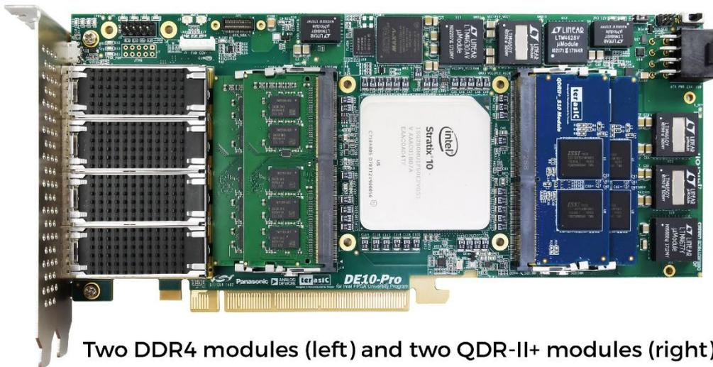
Two DDR4 modules (left) and two QDR-II+ modules (right)
