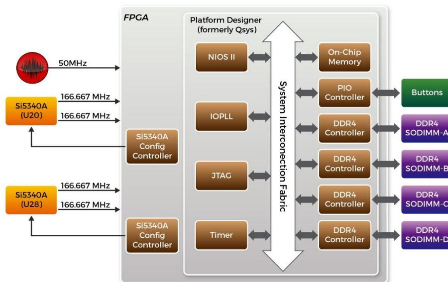
**Figure 6-2** Block diagram of the DDR4 Basic Demonstration
