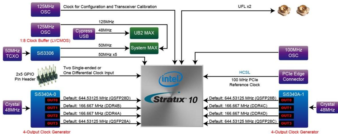
Figure 5-1 The clock tree of the DE10-Pro
