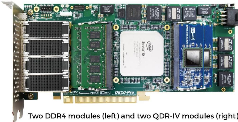
Two DDR4 modules (left) and two QDR-IV modules (right)
