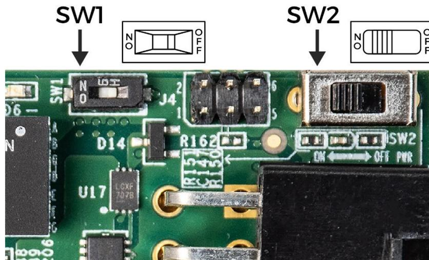
Figure 1-2 Board Power Control Switches
