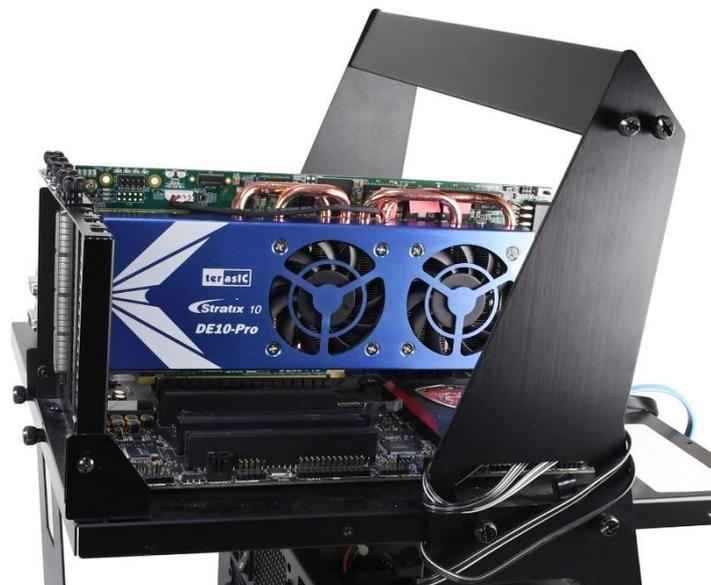
Figure 7-9 FPGA board installation on PC
