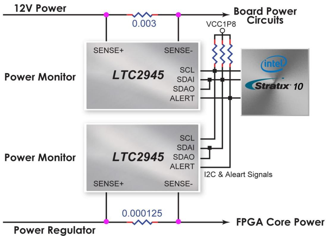
Figure 2-10 Connections between the Power Monitors and FPGA
