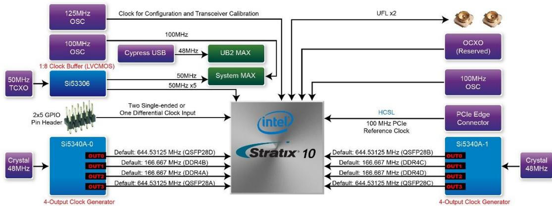
**Figure 2-11** Clock circuit of the FPGA Board
