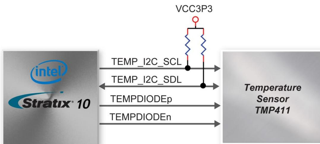
**Figure 2-8 Connections between the temperature sensor and FPGA**
