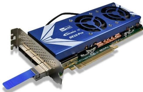
**Figure 9-7 Setup QSFP28 loopback fixture**
