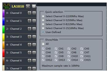
For example, if the first item is selected, the channels 0-2 would be enabled automatically, and the maximum sampling rate is 100M. If you select "user defined", the channel settings behavior is like what we just mentioned.
