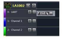
After the trigger is set and the button "start" is pressed again, if the trigger condition (falling edge) we have set have not appeared on channel 0, the logic analyzer would stay in wait state until the falling edge arrives. Then the device will sample and save the data, and upload the data to the computer for displaying and analyzing when the process is complete.
