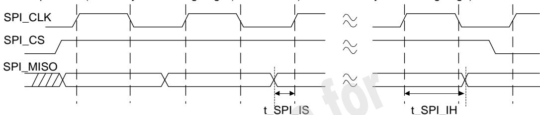
**Figure 3-11 SPI Timing**
