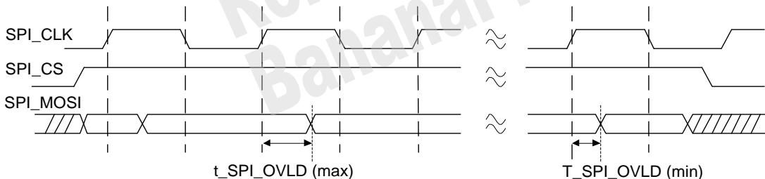
Read operation (Driven by clock rising edge (slave-device) and latched by clock rising edge)
