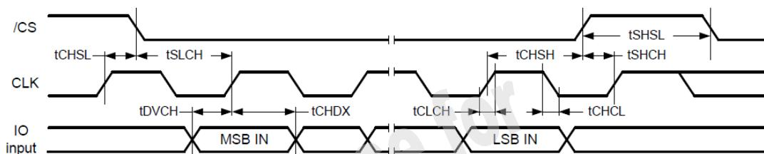
**Figure 3-17 SPI NAND Serial Input Timing**
