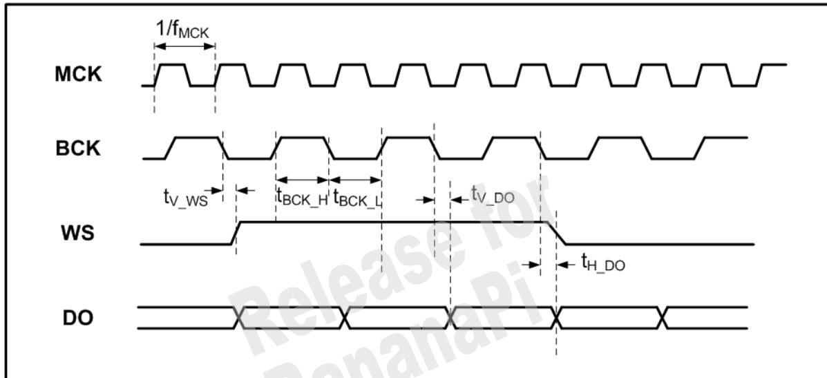
Figure 3-6 TDM master mode timing diagram
