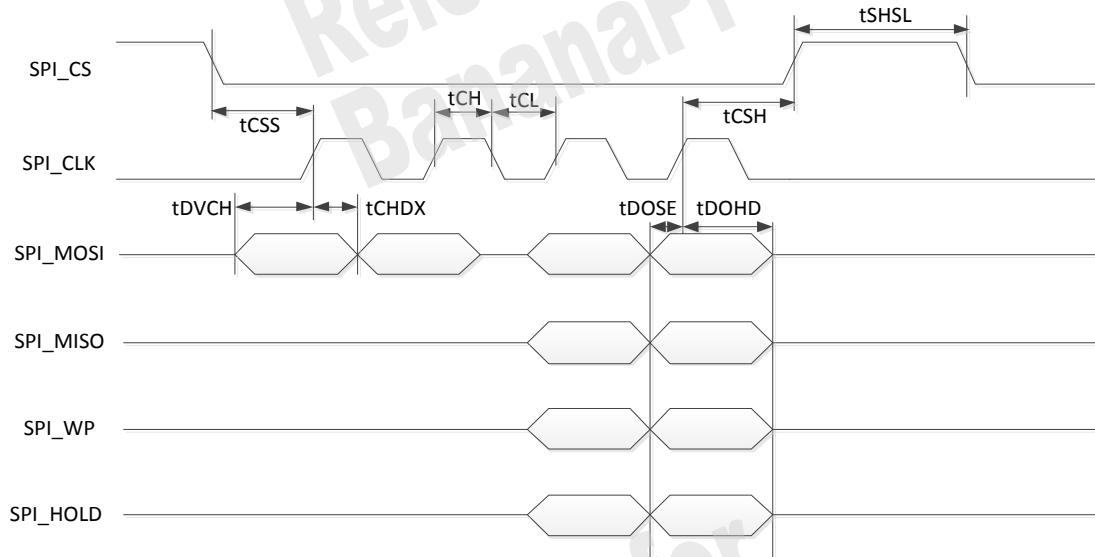
**Figure 3-12 SPI NOR interface timing**
