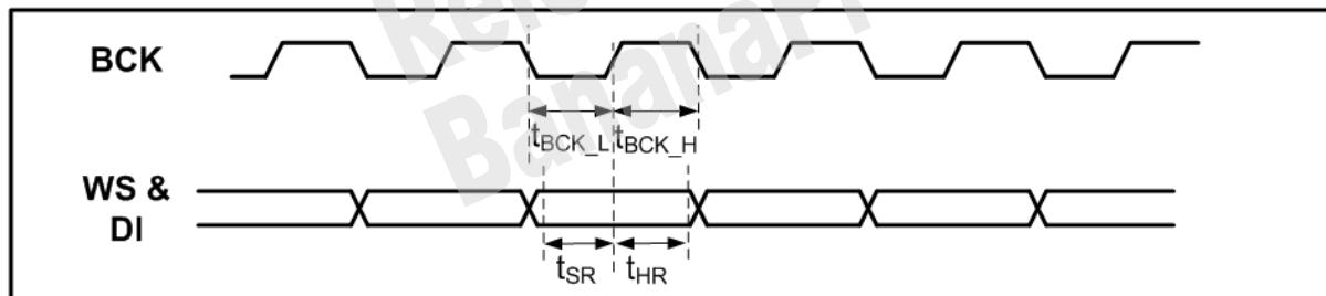
*Figure 3-5 I2S slave mode timing diagram*
