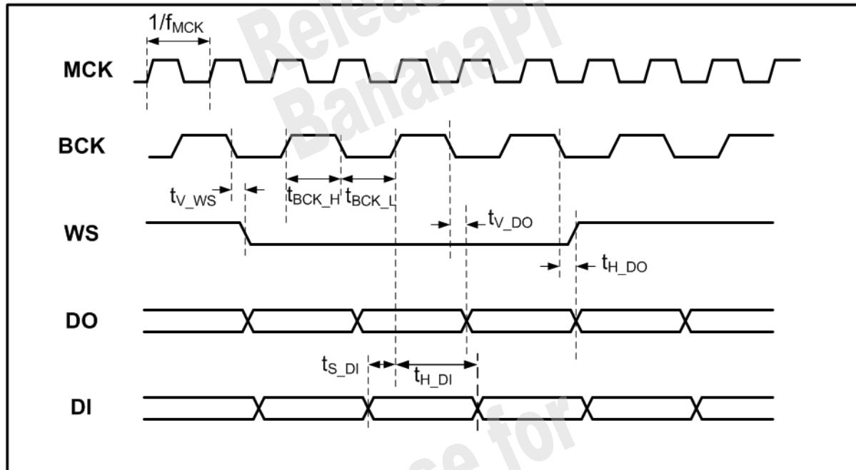
*Figure 3-4 I2S master mode timing diagram*
