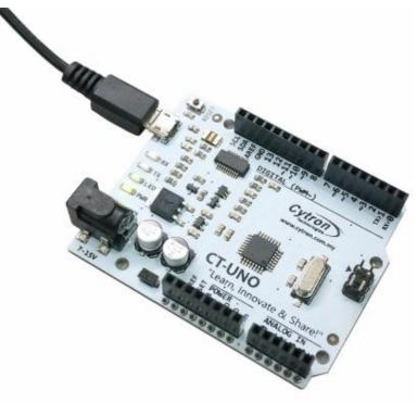
• If <u>CT-UNO</u> is powered with both 12V Power adapter and USB cable, it will automatically choose power from power adapter.
