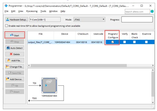
Figure 2-10 Program .sof file into the FPGA device
