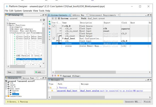
Figure 4-7 Rename and connect dual boot IP OK
