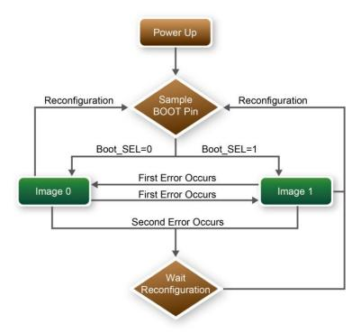
Figure 4-3 Remote System Upgrade Flow for MAX 10 Devices
