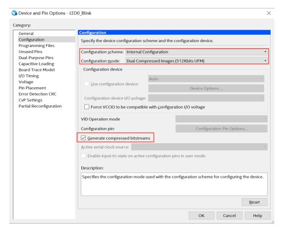
Figure 4-12 Set Dual Configuration Mode
