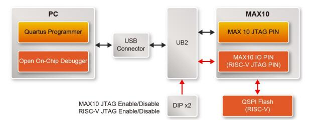
Figure 2-1 The JTAG configuration scheme
