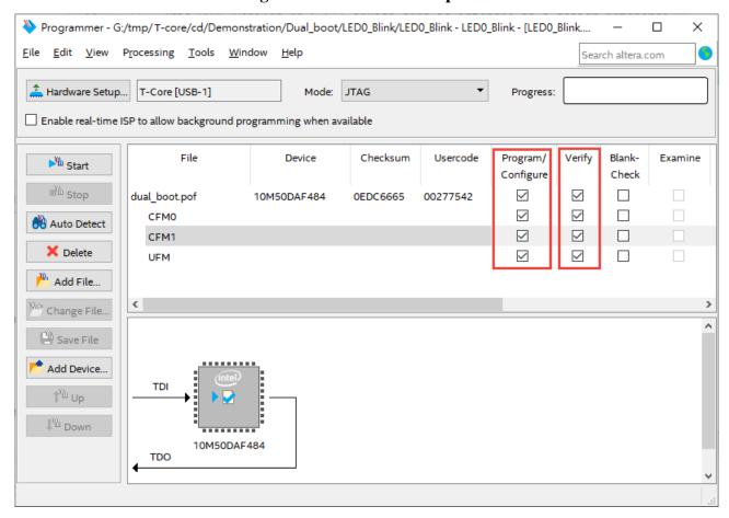
Figure 4-17 Programmer window with dual\_boot.pof file
