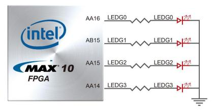
Figure 2-17 Connections between the LEDs and MAX 10 FPGA
