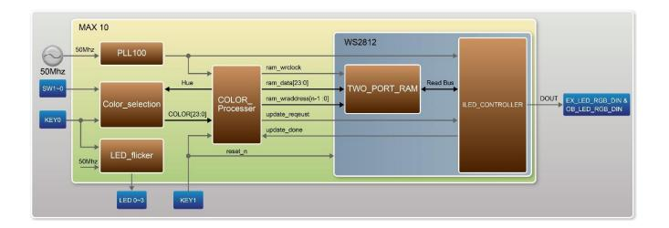
Figure 3-1 Block diagram of the Default demo
