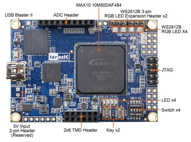
Figure 1-2 Development Board (top view)
