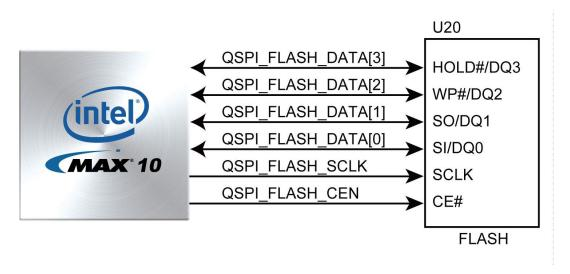
Figure 2-26 Connections between MAX 10 FPGA and QSPI Flash
