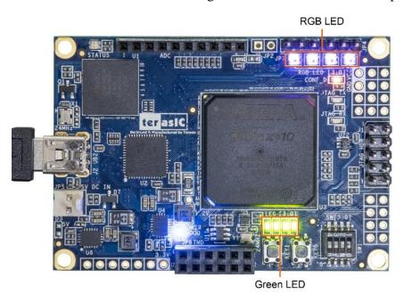
Figure 3-2 On-Board Green LED and RGB LED display
