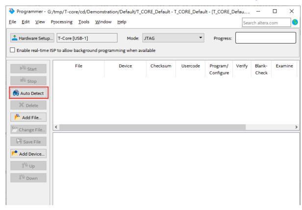
Figure 2-5 Detect FPGA device in JTAG mode
