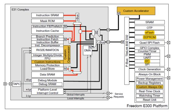
Figure 3-12 Top-Level Block Diagram of the E300 platform
