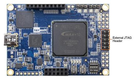
Figure 5-1 The external JTAG header of the T-Core board
