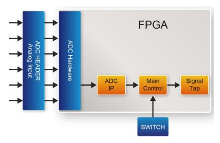
Figure 3-8 Block diagram of the ADC measurement demonstration
