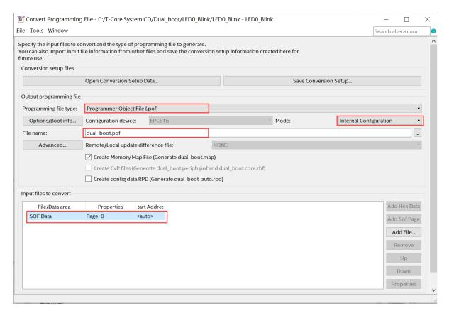
Figure 4-14 Dialog of Convert Programming Files and setting
