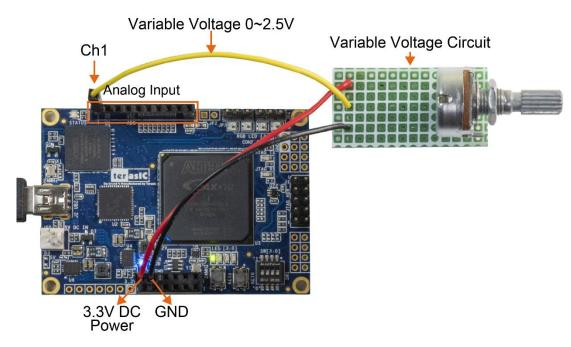
Figure 3-10 Connect analog source to the analog input
