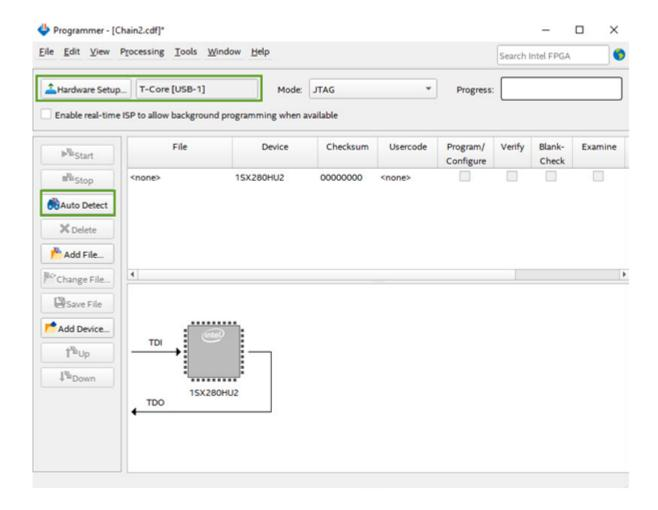
Figure 5-6 Using T-Core board to program the DE10-Pro
