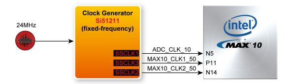
Figure 2-13 Clock circuit of the FPGA Board
