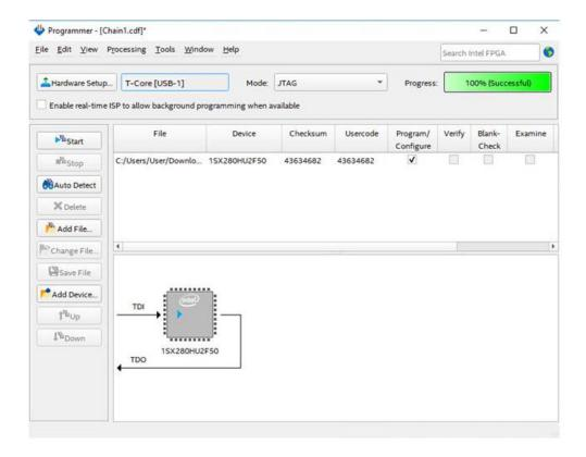
Figure 5-7 Using T-Core board to program the DE10-Pro
