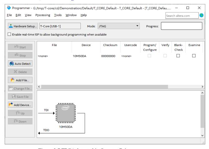
Figure 2-7 FPGA detected in Quartus Prime programmer
