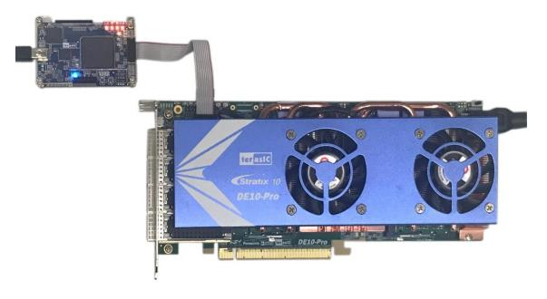
Figure 5-2 Using T-Core board as an USB Blaster II cable
