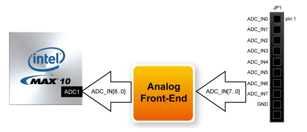
Figure 2-25 Connections between the Arduino Analog input and MAX 10 FPGA
