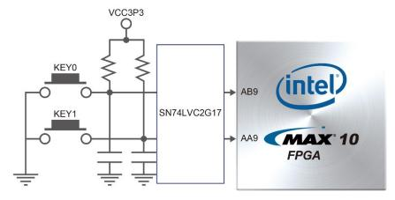
Figure 2-14 Connections between the push-button and MAX 10 FPGA
