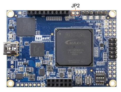
Figure 4-1 JP2 position on the T-Core board
