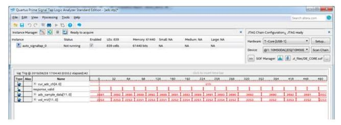
Figure 3-11 Signal Tap Logic Analyzer displays the measured channel and voltage
