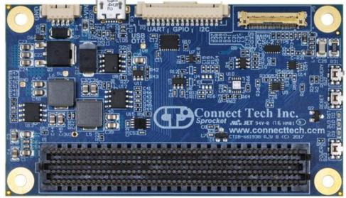
Recovery Switch (SW2) Reset Switch (SW1) LEDS (5V, 3V3, Reset) Power Switch (SW3)
