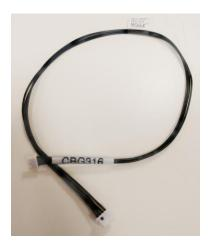
The CBG316 Fan cable allows for a connection to the FAN connector on CTI Jetson™ TX2/TX2i/TX1 carriers. The customer can use the cable asis, or modify the length and fan termination to easily connect any fan within their application. This offers the flexibility to use this cable in a wide variety of applications.
