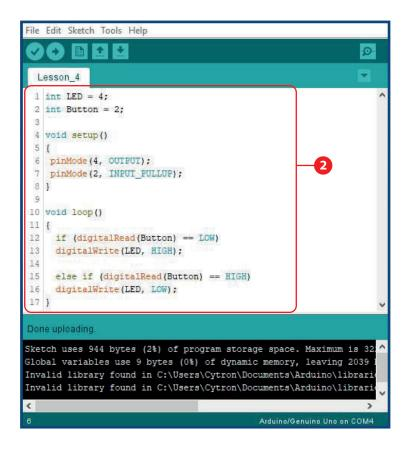
Push button act as a digital input device. Maker UNO is able to sense 2 states for digital input, i.e. HIGH and LOW. Push the button and the LED will turn ON!
