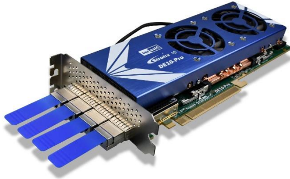
Figure 9-2 QSFP28 Transceiver Loopback Test in Progress
