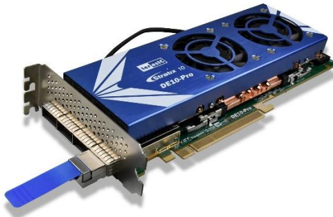
Figure 9-7 Setup QSFP28 loopback fixture
