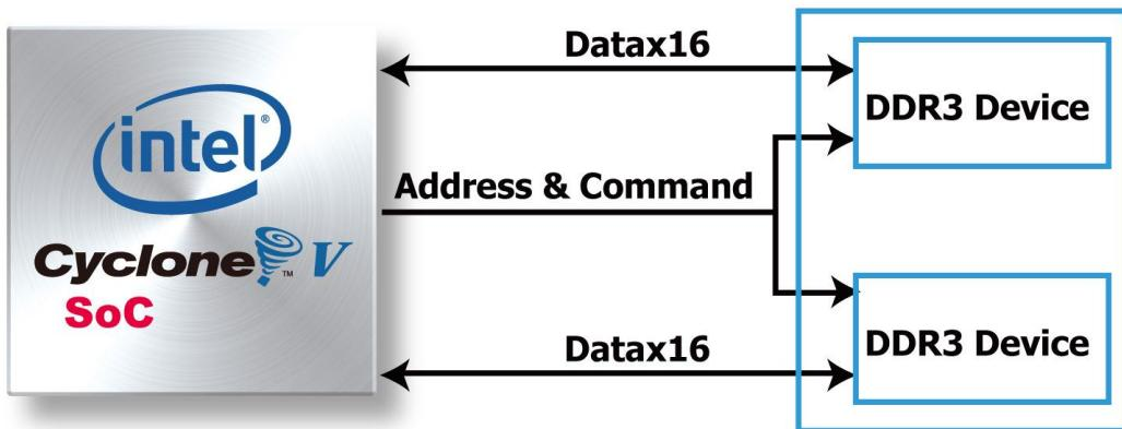
**Figure 4-5** Connections between the HPS and the DDR3
