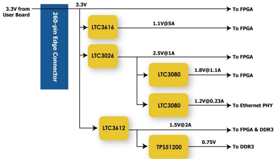
**Figure 2-4 Power Tree of the TSoM Module**
