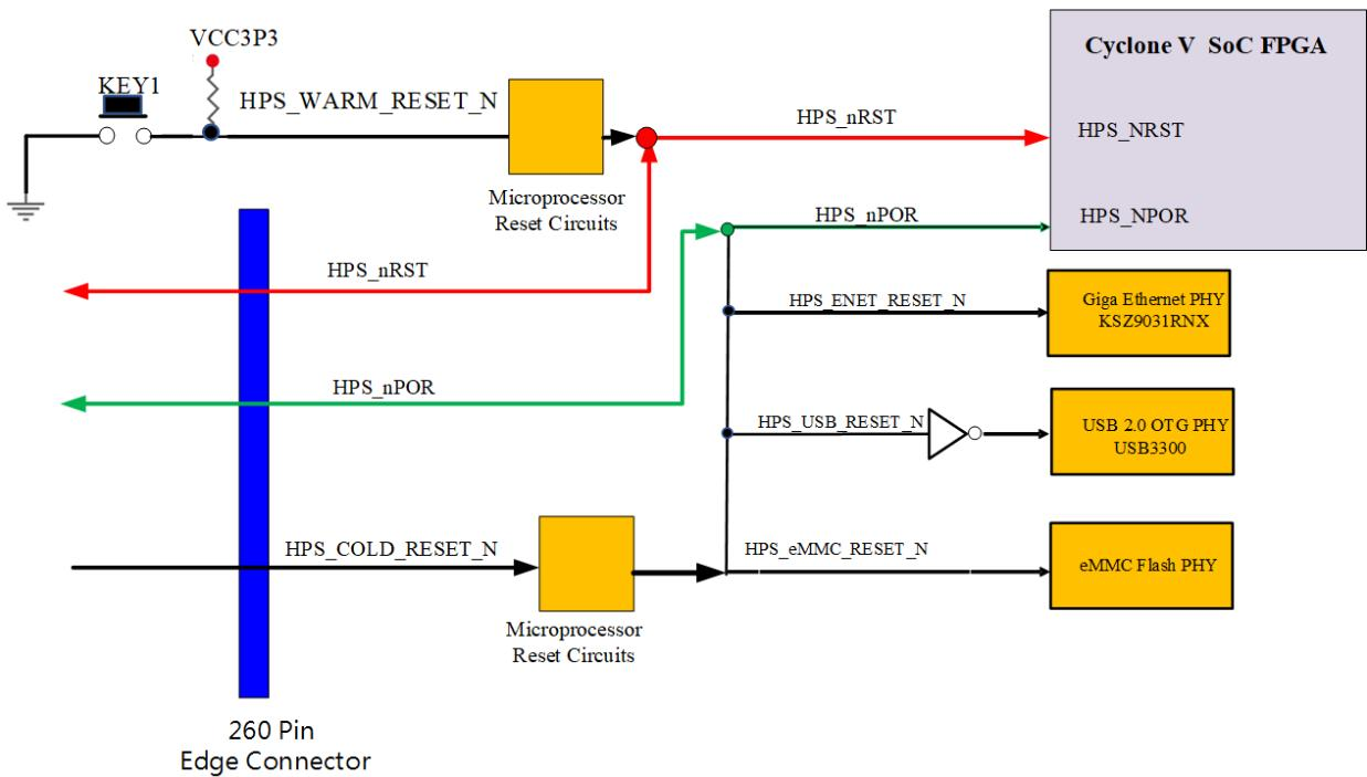
**Figure 3-11 Reset System of the TSoM Module**
