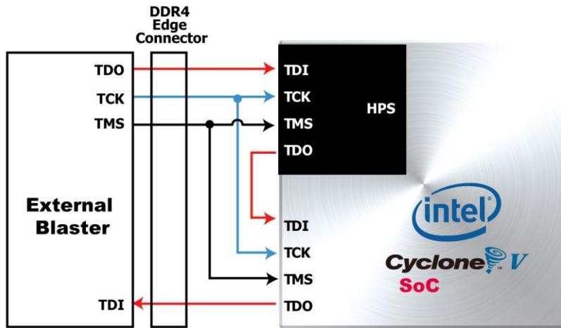
**Figure 3-4 JTAG Interface on the TSoM Module**
