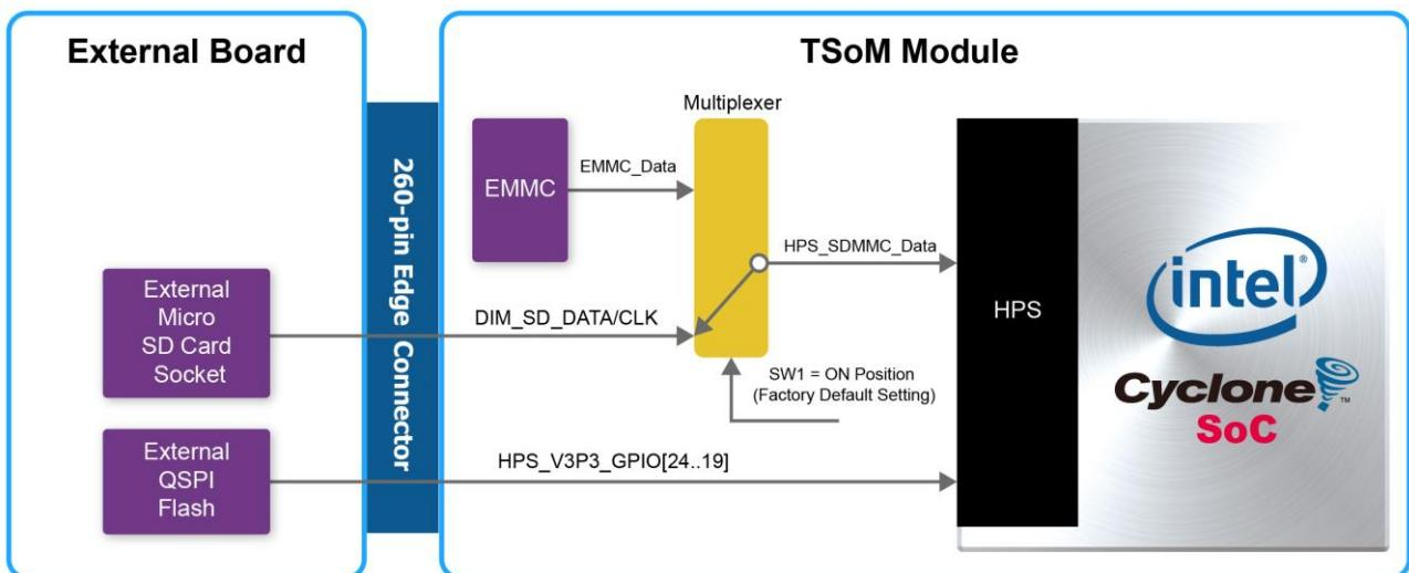
Figure 3-6 Boot Source on the TSoM Module
