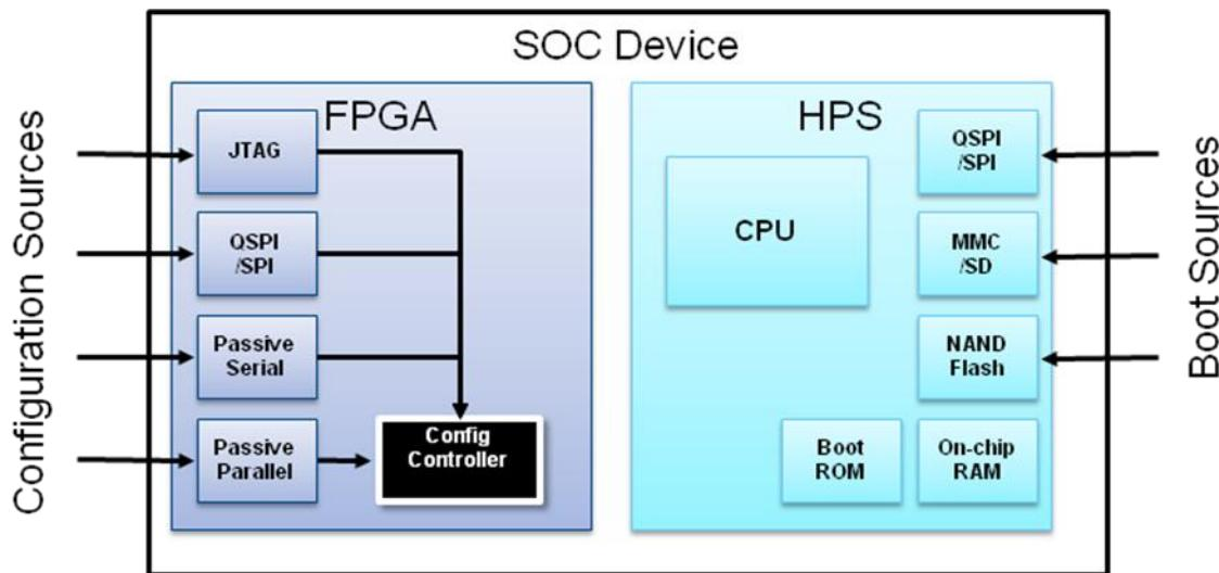
Figure 3-1 Independent FPGA Configuration and HPS Booting
