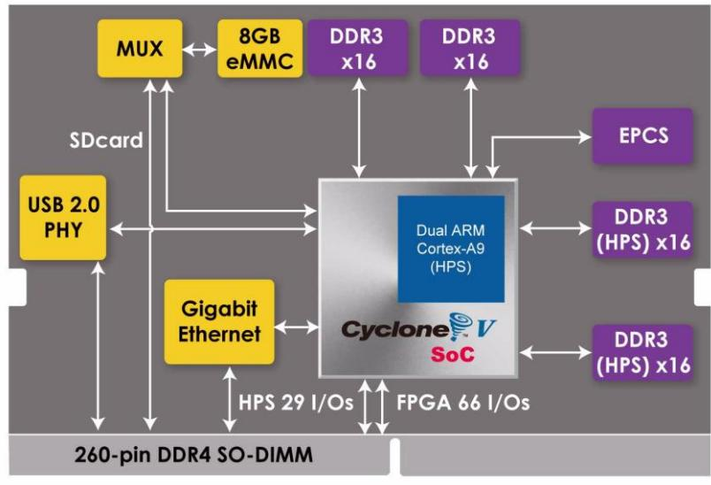
**Figure 2-2 Block diagram of the TSoM Module**
