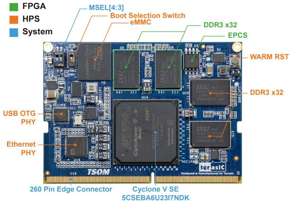
Figure 2-1 Mechanical Layout of the TSoM Module
