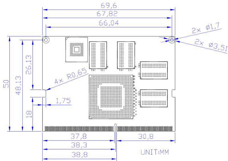
**Figure 2-3 Mechanical Layout of the TSoM Module**
