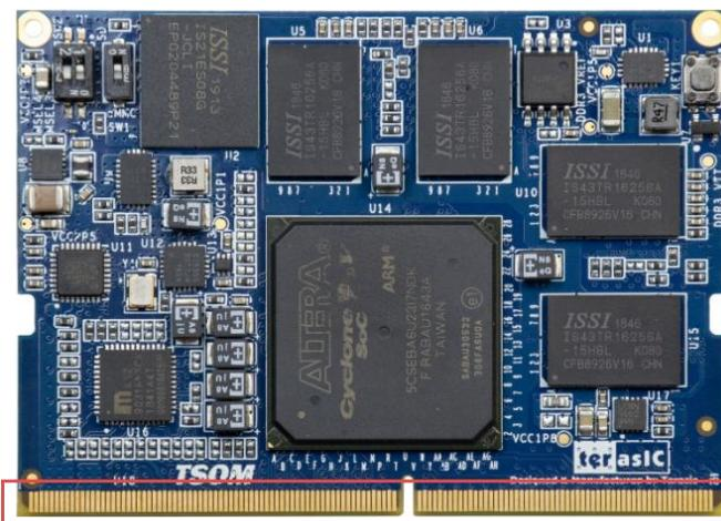
**Figure 3-12 260-pin edge connector on the TSoM module**
