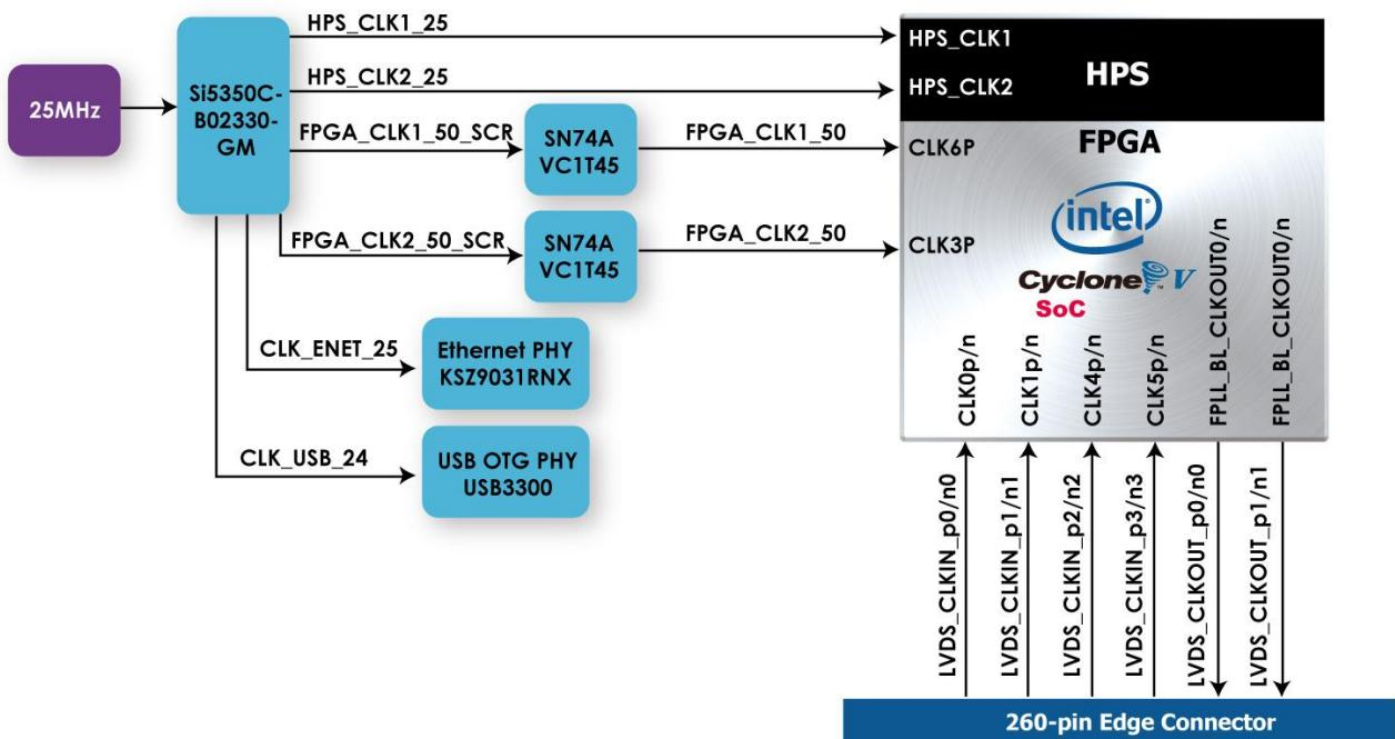
Figure 3-10 Clock System of the TSoM Module
