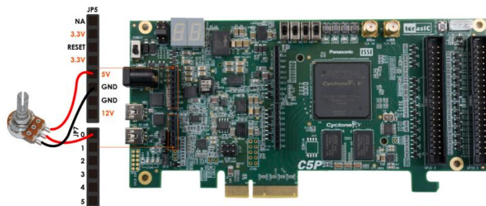
Figure 5-20 ADC Reading Demo hardware setup
