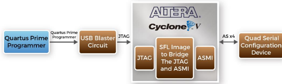
Figure 3-8 Programming a quad serial configuration device with SFL solution
