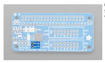
The MCP23017 has interrupt capabilities. There are two IRQ pins (INTA and INTB) you can solder a wire to, if you want to have a quick way of telling if any of the GPIO's changed.
