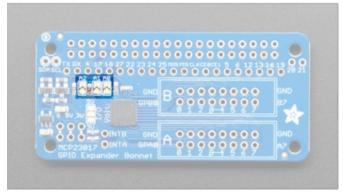
By soldering closed the address select jumpers, you can change the address from 0x20 to 0x27. This allows up to 8 bonnets for 128 total GPIO.
