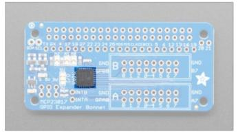
The MCP23017 GPIO expander chip converts Python code into pin instructions.
