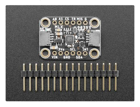
Comes as a fully assembled and tested breakout board with a small piece of header for use with a breadboard. As if that weren't enough, we've now also added <a href="SparkFungwiic">SparkFungwiic</a> (https://adafru.it/Fpw) compatible <a href="STEMMA QT">STEMMA QT</a> (https://adafru.it/Ft4) connectors for the I2C bus so you don't even need to solder the I2C and power lines. Just wire up to your favorite micro using a <a href="STEMMA QT">STEMMA QT</a> adapter cable. (https://adafru.it/JnB) Th
