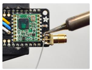
reason) Edge-Mount connector with 1.6mm spacing
