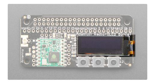
This bonnet comes with a 128x32 pixel OLED! The OLED is connected via I2C.
