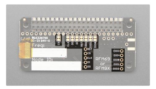
The two sets of pins here are broken out from the radio module. The defaults are:
