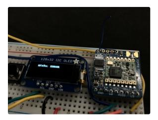
If the wiring of the radio module is incorrect - the display will show ERROR. Check over your wiring on the Wiring Page and re-run the test. You may also need to ensure the correct CircuitPython library is installed for the module.
