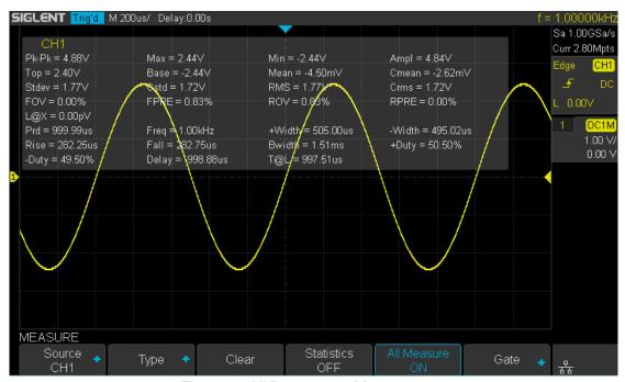
Figure 80 All Parameters Measurement
