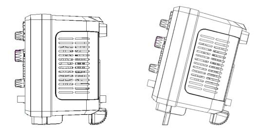
Figure 5 Adjust the Supporting Legs
