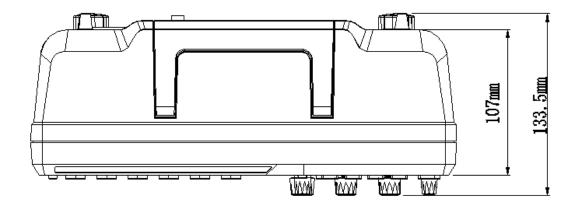
Figure 2 Top View (2-channel scope)
