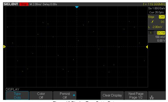
Figure 16 Display Type Set to Dots
