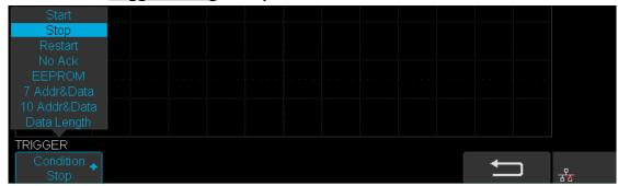
Figure 41 I2C TRIGGER Menu
