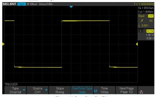
Figure 36 State DropOut Trigger
