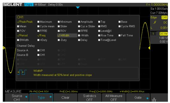
Figure 78 Select the Measurement Parameter
