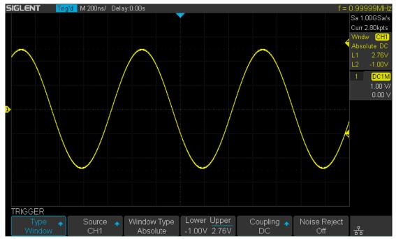
Figure 32 Absolute Window Trigger
