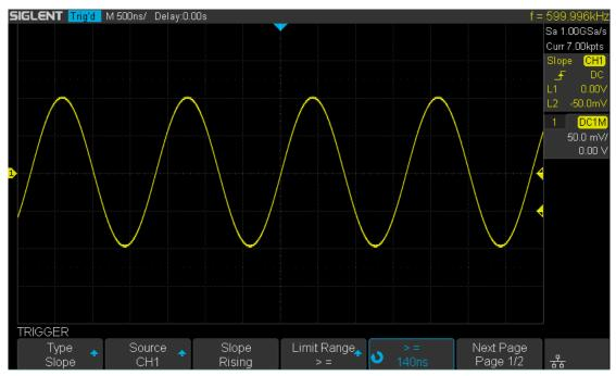
Figure 29 Slope Trigger
