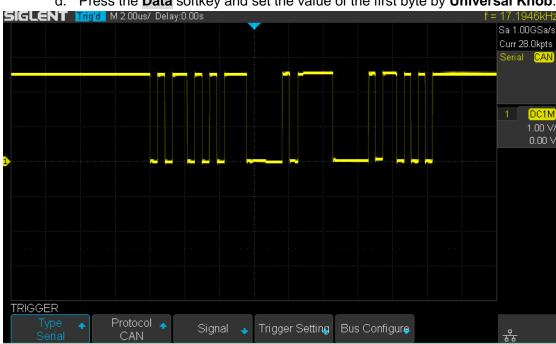
d. Press the **Data** softkey and set the value of the first byte by **Universal Knob**.
