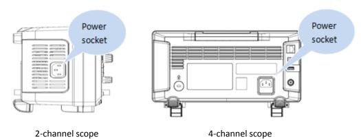
Figure 6 To Connect to Power Supply
