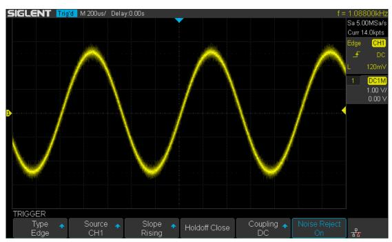
Figure 27 Turn on the Noise Reject
