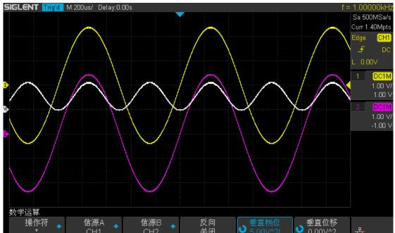
Figure 59 C1\*C2 Waveform
