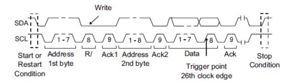
Data Length — When SDA data's length is equal to the value of Byte Length and address's length is the same as set value, the oscilloscope will be triggered. Byte length is in the range of 1 to 12 bits.
