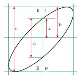
According to  $sin\theta=A/B$  or C/D (wherein,  $\theta$  is the phase deviation angle between the two channels and the definitions of A, B, C and D are as shown in the figure above), the phase deviation angle is obtained, that is:  $\theta=\pm arcsin(A/B)$  or  $\pm arcsin(C/D)$
