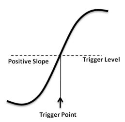
You can adjust the trigger level for a selected analog channel by turning the **Trigger Level Knob**.
