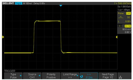
Figure 30 Pulse Trigger
