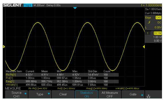
Figure 79 Added the Measurement
