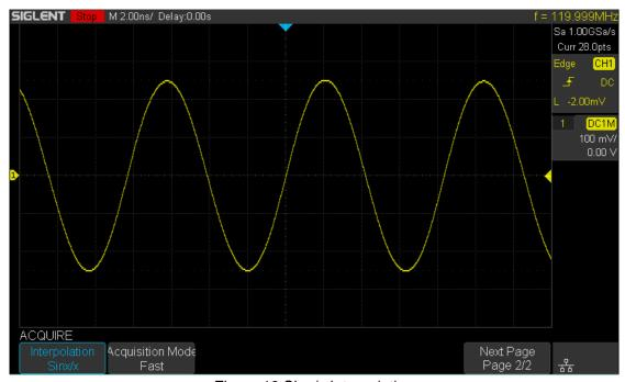
Figure 18 Sinx/x Interpolation
