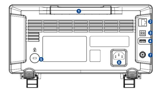
Figure 11 4-channel Scope Rear panel Overview
