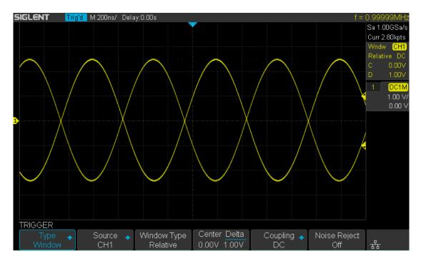
Figure 33 Relative Window Trigger
