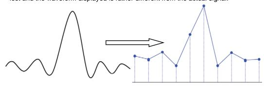
2. Waveform Confusion: when the sample rate is lower than twice the actual signal frequency (Nyquist Frequency), the frequency of the waveform rebuilt from the sample data is lower than the actual signal frequency. The most common aliasing is the jitter on fast edge.
