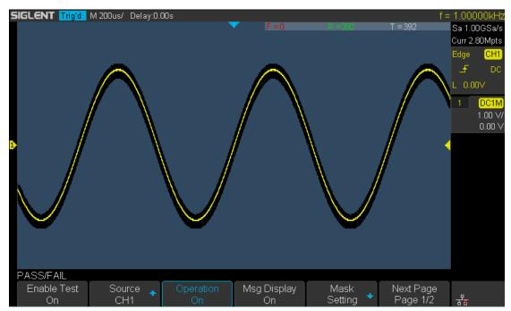
Figure 100 Pass/Fail Test
