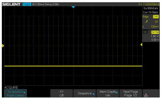
Figure 21 Pulse With 0.1% Duty, Peak Detect Mode
