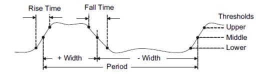
Figure 77 Time Measurements
