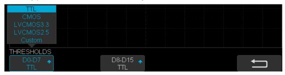
Figure 93 THRESHOLDS Function Menu
