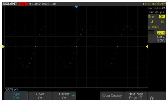
Figure 83 Dots Display
