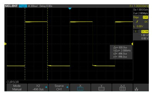
Figure 73 Measure Pulse Width
