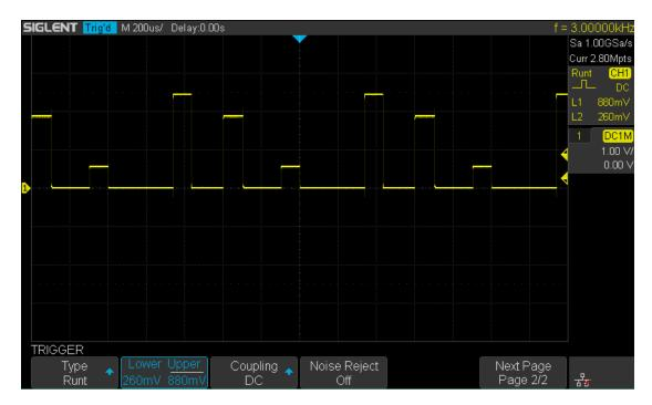
Figure 37 Runt Trigger
