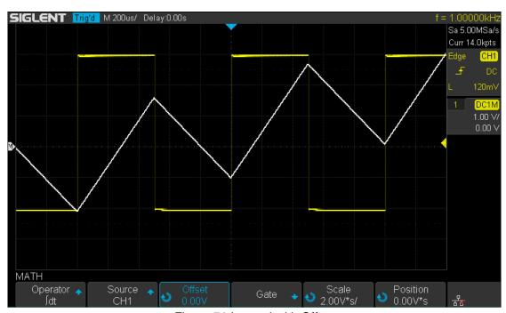
Figure 71 Integral with Offset
