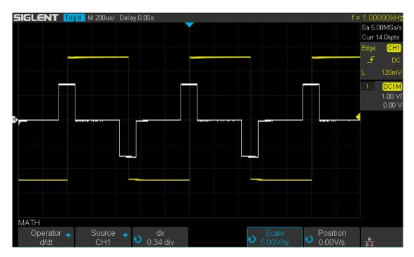
Figure 69 Difference Function Operation
