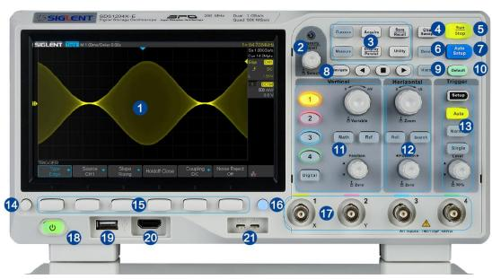
Figure 9 4-Channel Scope Front Panel Overview
