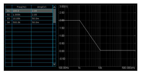
10. The Set Sweep and Set Stimulus in Vari-level editor are similar to that in the Simple sweep mode, but they are independently configured and do not affect each other. These options in Vari-level mode do not have frequency and amplitude input because they are specified in the spreadsheet. Press Set Sweep and then set Mode to "Decade", and set Points/dec to 20. The Set Stimulus remains default setting.
