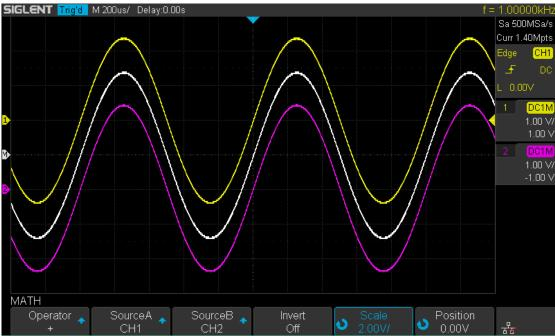
Figure 58 C1+C2 Waveform
