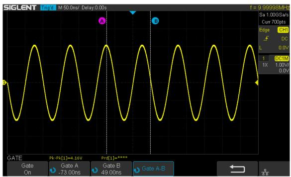
Figure 81 Gate Measurement
