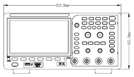
Figure 3 Front View (4-channel scope)
