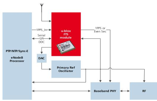
In this use case, the FTS device disciplines an external oscillator via an external DAC. During holdover the input
