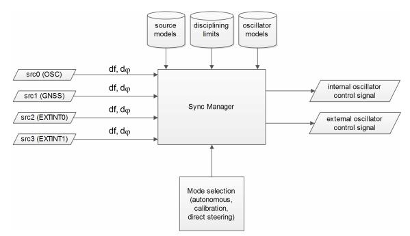
The user has the option to configure how the SMGR considers the external signals, e.g. time or frequency source, disciplined or not, etc... The user must also configure the uncertainty of the signals along with their nominal characteristics. One of the external signals may be configured as the feedback path of a disciplined external oscillator.
