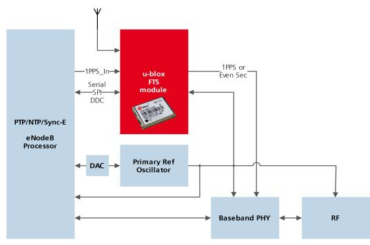
The frequency offset of the external oscillator is measured by the FTS device and communicated to the host which can then make any corrections necessary. The FTS device also generates a PPS phase reference internally (with no guarantee of coherence with the external oscillator). During holdover, the phase of 1PPS signal is maintained using either the primary reference oscillator or the 1PPS\_In signal, according to their respective uncertainty.
