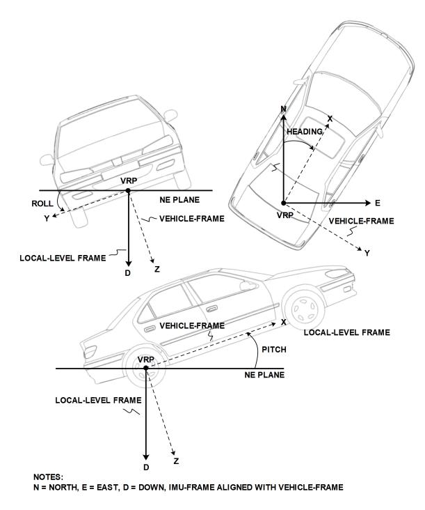
The order of the sequence of rotations around the navigation axes defining the vehicle attitude matrix in terms of vehicle attitude angles is illustrated below:
