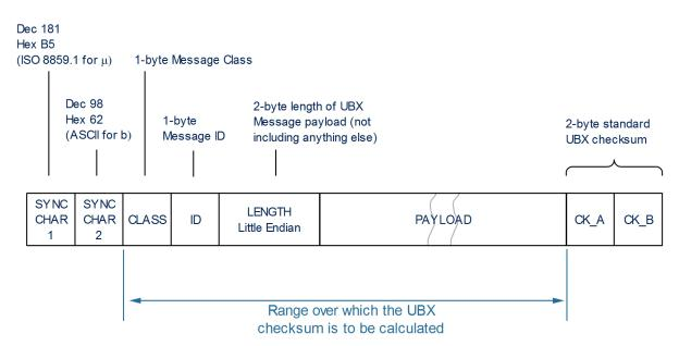
The checksum algorithm used is the 8-Bit Fletcher Algorithm, which is used in the TCP standard (<u>RFC 1145</u>). This algorithm works as follows:
