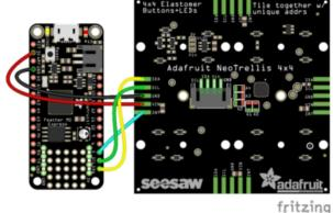
Wiring is easy, solder the four VIN GND SDA SCL pads to wires and then connect to your CircuitPython device
