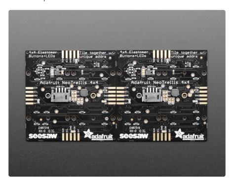
Perfect for your next cool interface, MIDI instrument, control panel...whatever could benefit from beautiful diffused colorful buttons. For fast connection to a single board, we include a JST-PH 4-pin connector that will give you power+data access. It's Grove compatible (the cable fits, even though its not the exact same connector), or you can use a JST-PH 4 pin cable (https://adafru.it/CzH).
