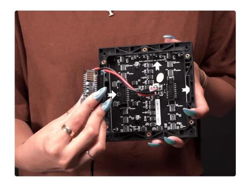
Either way you decide to go, you can plug a 5V DC power pack into the 2.1mm DC jack. That 5V is polarity protected and then output on the other side to a 5.08mm terminal block. An onboard regulator will provide 3.3V power to your Feather so you don't need a separate USB or battery, this makes for a very compact build!
