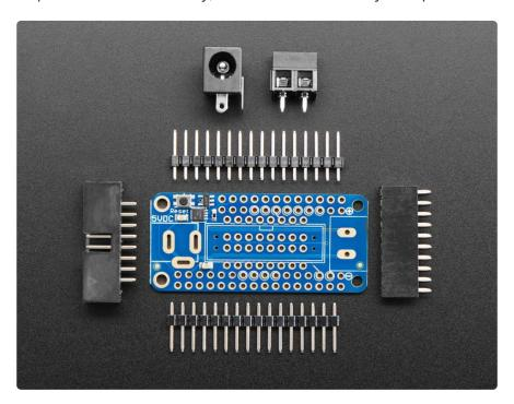
Each order comes with one FeatherWing PCB with surface mount parts attached, a 2x8 IDC header, a 2x10 female socket, 2.1mm DC jack, 5.08mm terminal block, and some male header. You may also want some Feather stacking headers (https://adafru.it/oAP) or female headers (https://adafru.it/waW) depending on how you plan to attach/stack your Feather.
