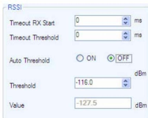
Figure 2-25. RSSI data entry area (Auto Threshold OFF)
