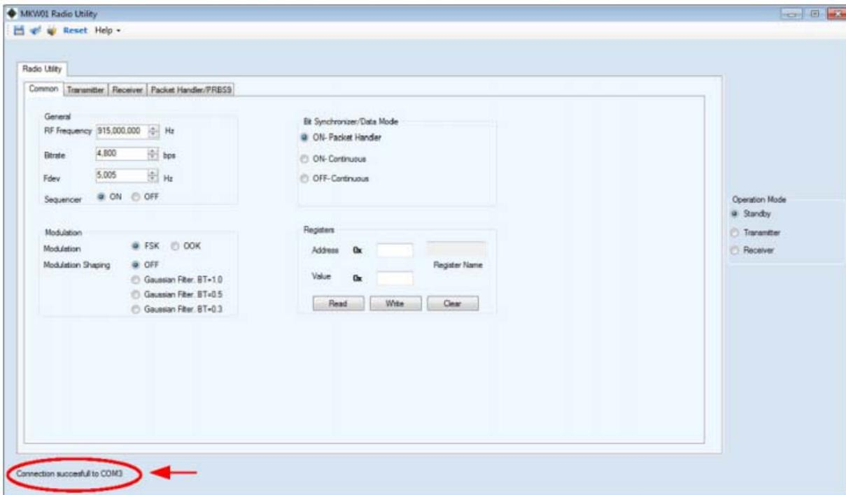
**Figure 2-3. Radio Utility successful connection**
