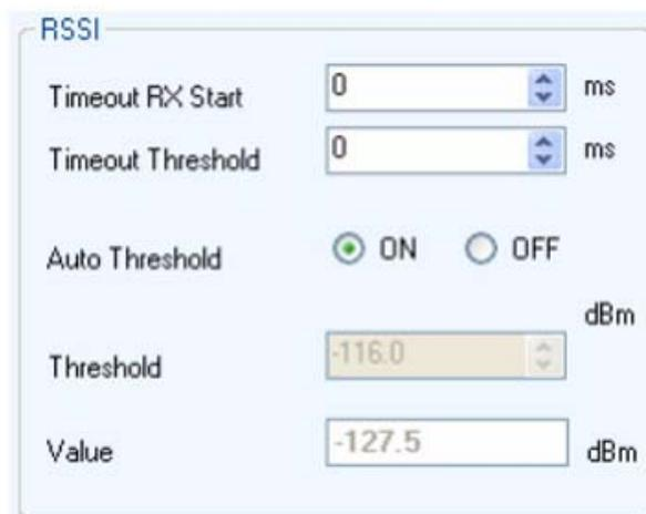
**Figure 2-24. RSSI display area (Auto Threshold ON)**
