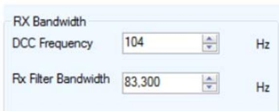
Figure 2-20. RX Bandwidth display area
