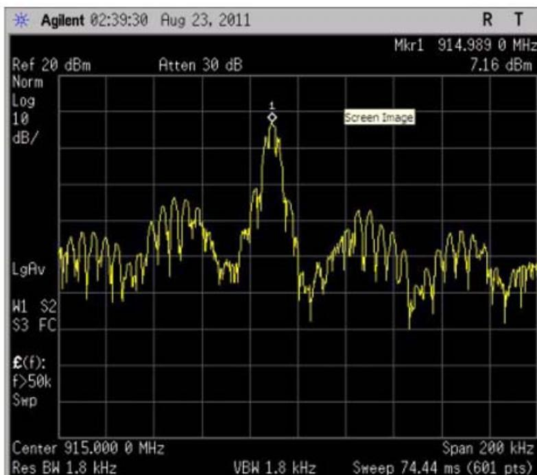
Figure 2-32. Transmit with modulation OOK (filtering with fcutoff = BR)
