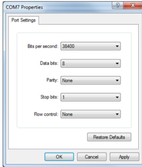
**Figure 1-10. COM port setup**
