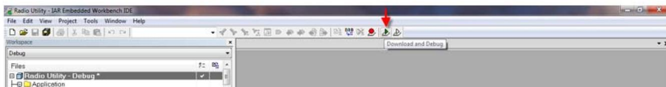
**Figure 1-7. Downloading and debugging an application in IAR**
