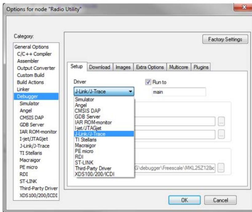
**Figure 1-5. Selecting the debugger driver**
