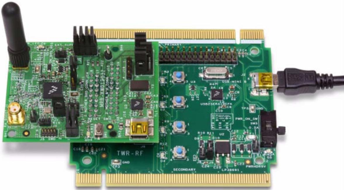
**Figure 1-13. MRB board mounted on the TWR-RF board**
