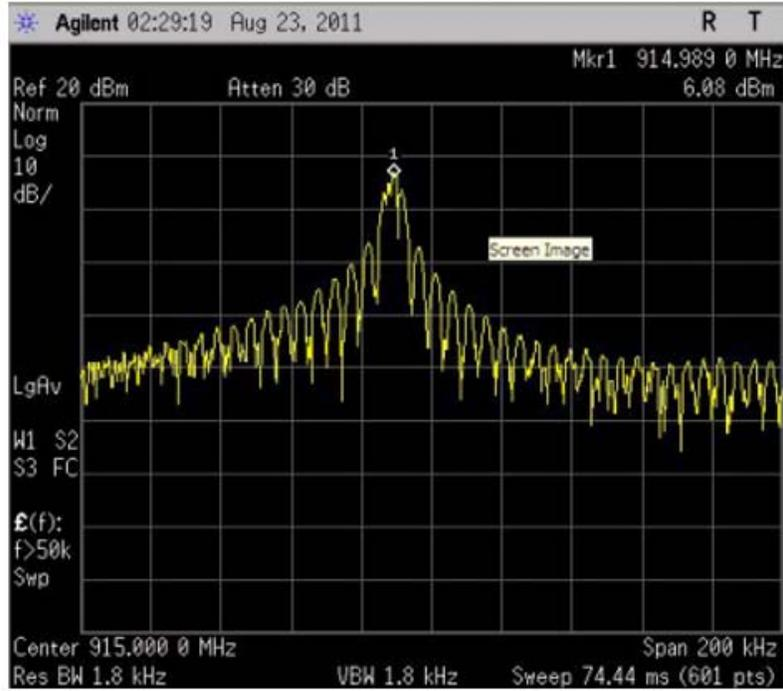
Figure 2-31. Transmit with modulation OOK (OFF)
