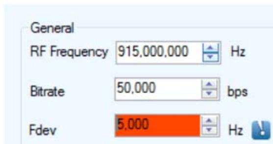
**Figure 2-8. General display area highlighting an invalid parameter**
