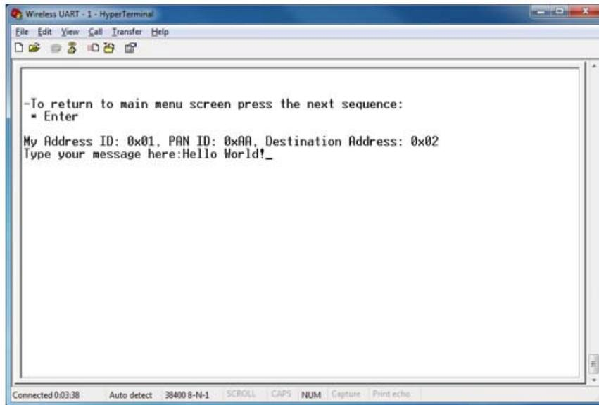
Figure 3-6. Typing message in board 1
