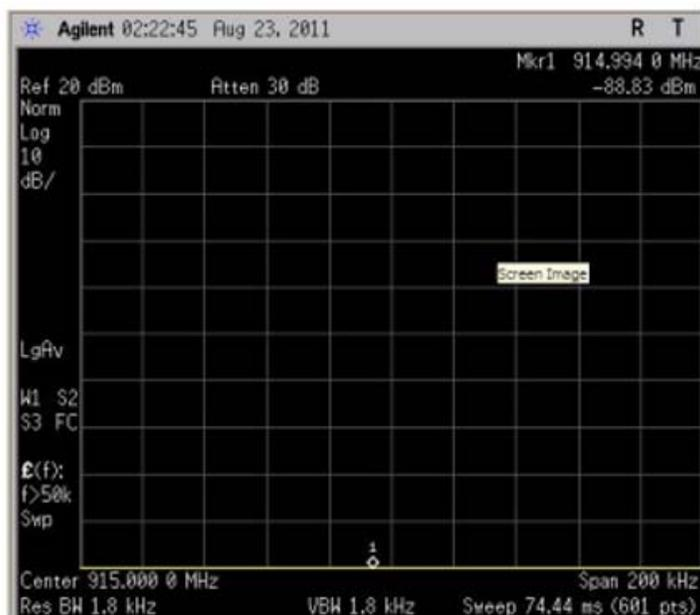
Figure 2-27. Standby mode spectrum analyzer capture
