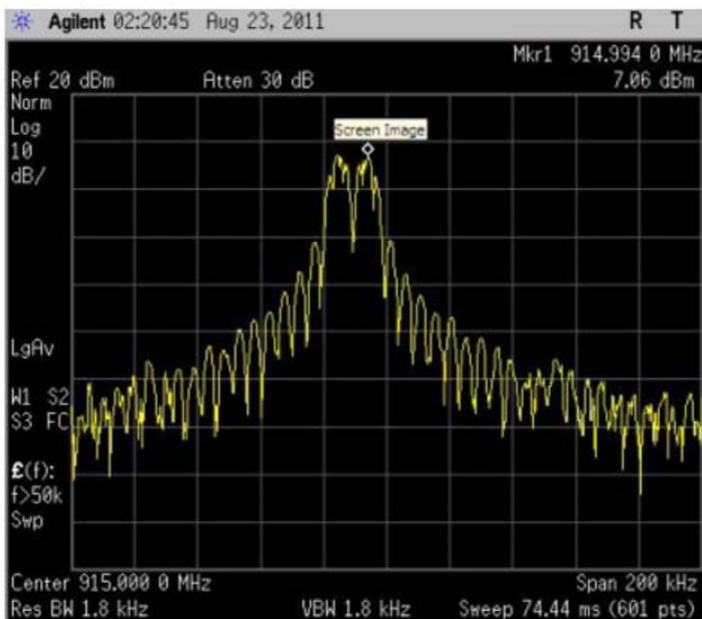
Figure 2-30. Transmit with modulation FSK (gaussian filter BT = 1.0)
