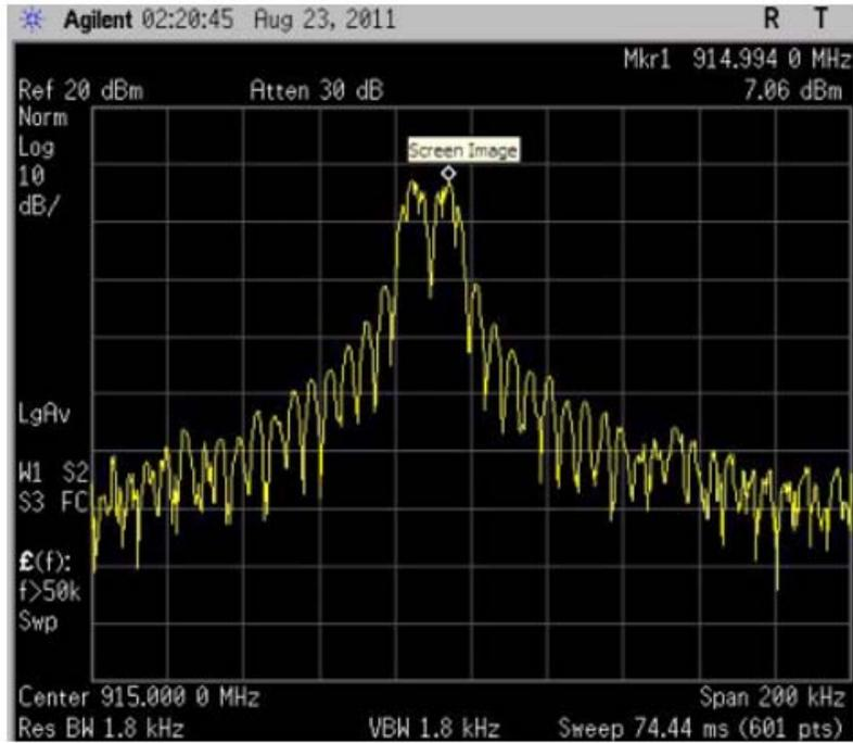
Figure 2-29. Transmit with modulation FSK (with modulation shaping OFF)
