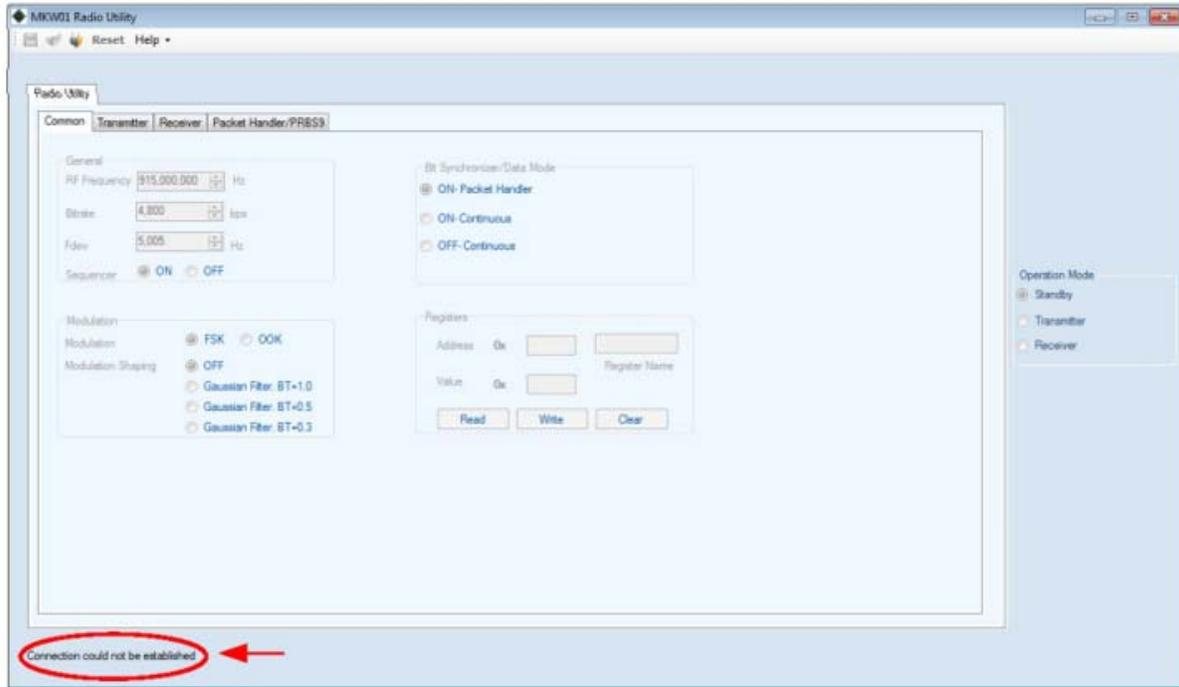
Figure 2-4. Connection not established
