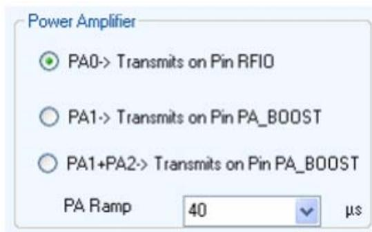
Figure 2-17. Power Amplifier display area
