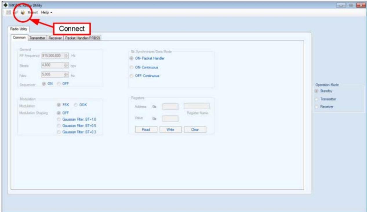
**Figure 2-2. Main window Connect button**
