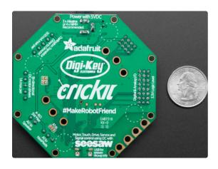
There are circular markings on the bottom of Crickit for four mounting pads (Adafruit ID 550 (https://adafru.it/dLG)) if you would like to use the board on a surface and protect the surface and bottom of your Crickit.
