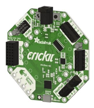
Watch out, the CircuitPlayground Express (CPX) can go on 'backwards' and it won't work. Make sure the USB connector on the CPX is right below the DC jack, and the labels on the silkscreen of the Crickit match the ones on the CPX! See the images below!
