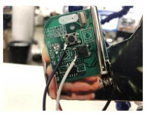
For the remote, we soldered four wires
