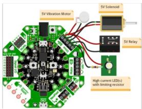
In addition to servos and DC motors, you may find you want to drive other high-power electronics like relays, solenoids, powerful LEDs, vibration motors, etc. Some of these devices are motor-like and need a kick-back protection diode, so having a proper driver is important to avoid damage!
