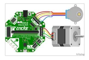
And the micro:bit can control stepper motors also when plugged into the micro:bit version of Crickit (micro:bit not shown for clarity).
