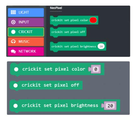
You can use the three special NeoPixel blocks in the **CRICKIT** block group extension to change the single NeoPixel on-board Crickit. They work just like the NeoPixel blocks under the **LIGHT** block group but just for the one Crickit pixel.
