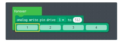
Then you can set the value from 0 (drive off) to 1023 (drive all the way on). If you want to dim an LED or run a vibration motor at half power, use 512. For quarter power, use 256!
