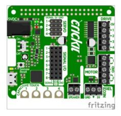
The Crickit HAT for Raspberry Pi uses the standard Pi 40 pin header (at top in the picture at left) to plug onto the Pi expansion header.
