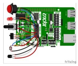
The Signals block on the Crickit HAT for Raspberry Pi gives you 8 bidirectional general purpose input/output (GPIO) (analog/digital) ports.
