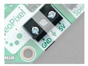
Connect the capacitor using the **NeoPixel** terminal blocks. The **5V** and **GND** lines are shared across the board so even if its a DC motor or servo causing the issues, this will help!
