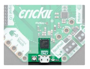
The seesaw chipset is the programmed ATSAMD21 processor in the south section of the board. It comes with its own parts too
