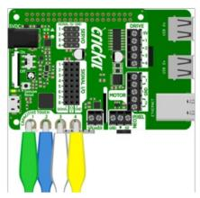
The four capacitive touch pads on the Crickit HAT for Raspberry pi are conveniently on the edge and vave nice holes for clipping alligator clips onto.
