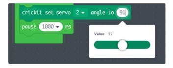
Although the angles range from 0 to 180, servos may have different ranges depending on the make and model. Also, each servo is a little different, so you may not get precisely the same angle even if its the same servo! Tweaking/adjusting the angle may be necessary.
