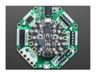
Once you have the Circuit Playground Express lined up correctly, use the remaining screws to attach the boards together. Start with one screw into one standoff, say GND, leave it loose a bit, then put in the VOUT screw, loose, then the others loosely. Ensure things are lined up, then carefully tighten each screw. Again, a firm connection but not overly tight.
