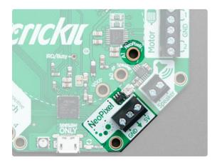
Blinky lights will make your robot fun and fashionable. And we've made it really easy to add NeoPixels (WS2812/WS2811/SK6812 chipsets) to your project. The Crickit has a 3-terminal block connector with **Ground**, **Signal** and **5V** power. The signal line has a level shifter on it so it will be 5V logic level, for nice clean signals.
