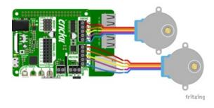
Likewise you can drive two stepper motors with the Crickit HAT for Raspberry Pi. One on the Motor ports, one on the Drive ports.
