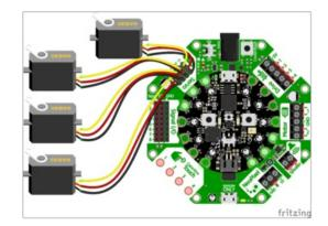
You can plug up to four servos in the **Servo** block of Crickit. The pin spacing is just right for servo connections.
