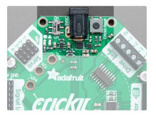
Your project start here, where power comes into the Crickit and is then used to control various motors and parts. We cover the various ways you can power your Crickit in the next section, since there's a lot of flexibility depending on the budget, portability and complexity of your project.
