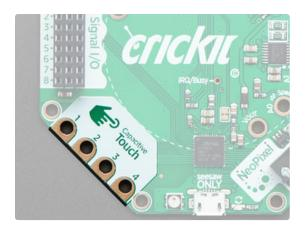
Capacitive touch sensing allows you to add human-triggered control to your robot. When you touch the pad (either directly or through an alligator clip, copper tape or conductive ink) the Crickit can detect that signal. We give you four capacitive touch inputs with alligator/croc clip compatible PCB pads.
