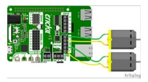
DC motors are controlled by 4 PWM output pins, the 4 PWM pins let you control speed and direction. And we'l use our **seesaw\_Motor** library to help us manage the throttle (speed) and direction for us, making it very easy to control motors
