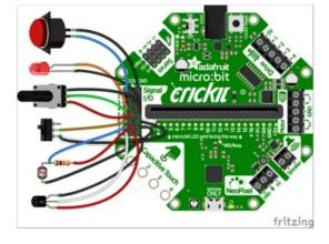
The 8 GPIO pins on the Crickit are in the Signals block of pins. You have the 8 data pins, each input/output, 3.3v logic, analog or digital.
