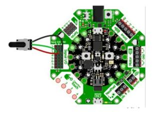
You can also read analog values like from a potentiometer or sensor.
