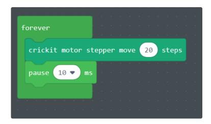
You'll see the motor shaft slowly turning in the "positive" direction. If you use a bit of solid tape on the stepper's shaft as a small flag, you can see the rotation better. If the rotation is in the wrong direction, use a negative value for the number of steps, re. -20.
