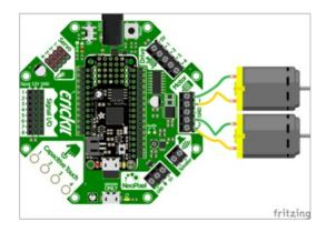
The Feather Crickit connections for the Motor terminals is shown at left.
