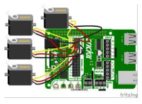
The Crickit HAT for Raspberry Pi can also control up to 4 servos like other Crickit boards. Note the location of the Servo header block with 4 rows of three male pins.
