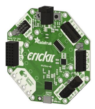
Another common issue we see is not having good power to the Crickit. Check that you have fresh batteries or a good 5V power supply. Also check the Crickit is on! There's an on/off switch next to the power jack
