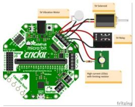
The Drives port provides the ability to drive higher current devices.
