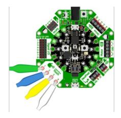
There's four capacitive touch pads you can use to detect human touch. They have big pads you can use to attach alligator/croc clips
