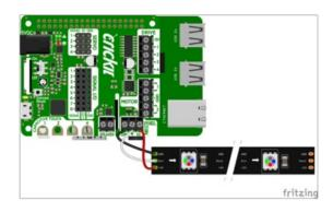
The Crickit HAT for Raspberry Pi has the NeoPixel block along the edge for easy wiring.
