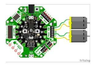
You get 2 independently-controllable brushed DC motor drives. Each motor can go forwards or backwards, with 8-bit speed control. There's a 5-pin terminal block to connect motors, 2 pins for each motor and a middle ground pin. (The ground pin is for some advanced techniques)
