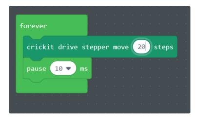
If you want to move the motor in the opposite direction, make the movement value negative, re. -20. The block takes positive and negative values.
