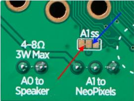
Turn the Crickit over and locate the jumper block on the bottom as circled in yellow in the first image.
