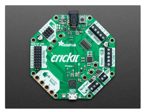
Since you'll be working with high-current devices, we wanted to have a good solid power supply system that minimizes risk of damage. The power supply has an <u>'eFuse' management chip</u> (https://adafru.it/Bfj) that will automatically turn off if the voltage goes above 5.5V or below 3V and has over-current protection at 4A. Every motor driver has kick-back protection. We think this is a nice and durable board for robotics!
