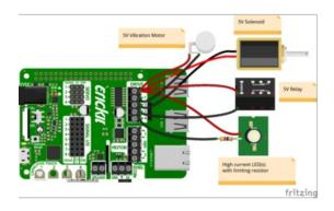
Crickit HAT for Raspberry Pi can also drive four devices via the Drive ports.
