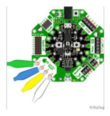
There are four capacitive touch pads you can use to detect human touch. They have big pads you can use to attach alligator clips to extend the pads' reach.
