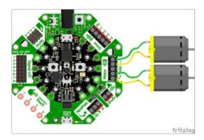
Connections from DC motors to the Circuit Playground Express Crickit is shown at left. There are two **Motor** drivers, labeled **1** and **2**.
