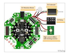
The **Drives** block on Crickit makes it super easy to connect higher current devices.
