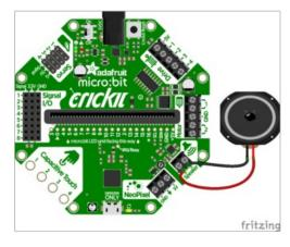
The micro:bit version of Cricket also has amplified audio output.
