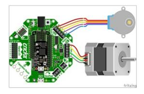
The Crickit with Feather uses identical connections with other Crickit boards to stepper motors.
