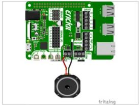
The Speaker block on the Crickit HAT for Raspberry Pi is easily to use, on the edge of the board. The onboard amplifier is very handy to provide audio for various projects.
