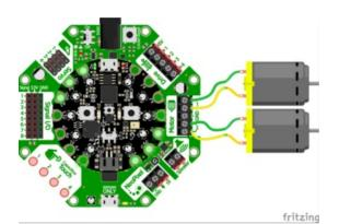
The hexagonal Crickets at left all have a similar Motor port which can drive two DC motors.
