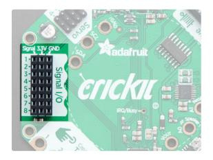
Sure you can drive servos and motors but sometimes you just want to blink an LED or read a button. The Crickit has an eight-signal port. You can use these as "general purpose" input/output pins. We solder a 3x8 female socket header in so you can plug wires in very easily. Each signal has matching 3V and Ground power pins.
