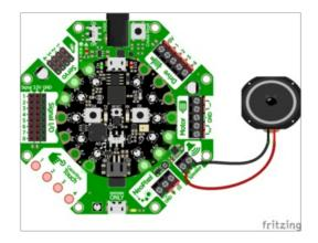
Crickit provides an amplified audio output via the **Speaker** block.
