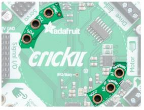
Using a Philips screwdriver and the provided screws, attach the standoffs to the six large holes on the inside ring of Crickit. There are three holes near the Adafruit logo and three more near the Neopixel and speaker outputs. You do not want to put the standoffs on the holes on the outside edge of Crickit - there are 8 mounting holes there but these standoffs are needed for the Circuit Playground Express.
