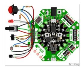
The **Signals** block on Crickit allows you to expand your general-purpose inputs and outputs (GPIO).
