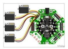
The Crickit gives you 4 slots for 4 independent servos. You can use micro, mini, standard, large size servos. Analog and digital work great. Continuous or 180-degree are OK. As long as you've got a servo with a 3-pin connector, you're golden.
