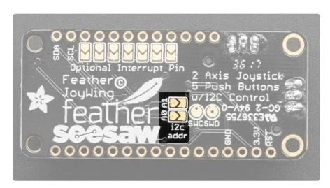
Because multiple featherwings of all kinds can be stacked, the I2C address can be changed if necessary. The Joy Featherwing's default I2C address is 0x49, but soldering jumpers A0 and/or A1 can change this:
