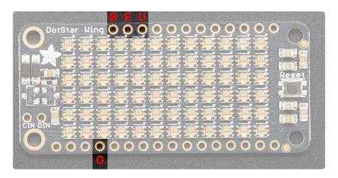
The Battery and Usb power pins are used to power the many DotStars. There's a lot of pixels and you can't really run them from the 3.3V regulator. Two 1A Schottkey diodes will automatically select whichever voltage is higher. That means, if USB is plugged in, you'll get  $^{\sim}5V$  USB power. If the feather is running off of battery power, say a LiPoly battery, you'll get 3.7-4.2V power. While this is a little lower than spec, DotStars are only a little dimmer.
