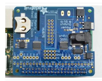
Check over your work so far, make sure each solder point is shiny, and isn't bridged or dull or cracked
