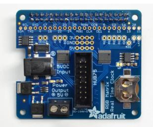
Place the connector in the slot so that the notched side is on the **left**
