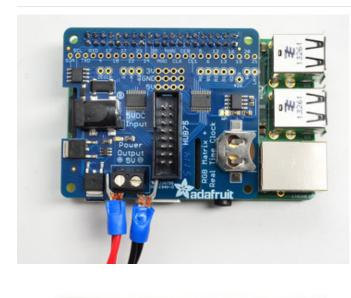
Plug the red wire into the + side, and the black wire into the - side.
