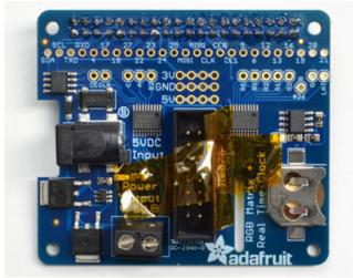
Use some tape to hold the IDC connector in place
