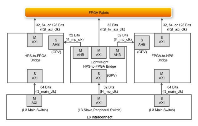
Figure 7-1 AXI Bridge Block Diagram
