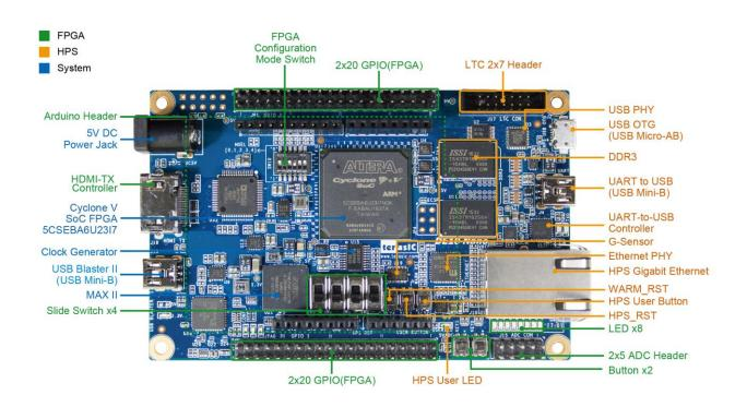
Figure 2-1 DE10-Nano development board (top view)
