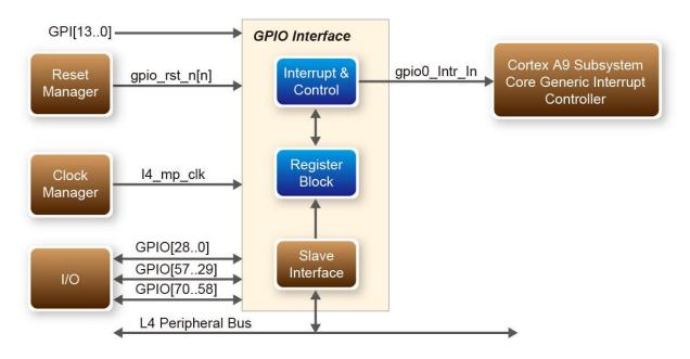
Figure 6-2 Block diagram of GPIO Interface
