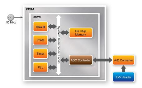
Figure 5-2 Block diagram of ADC reading
