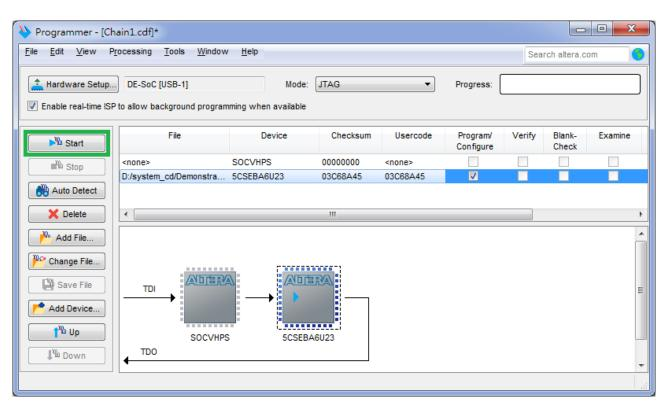
Figure 3-10 Program.sof file into the FPGA device
