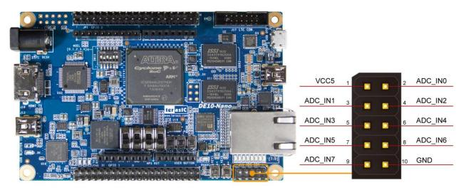
Figure 3-22 Signals of the 2x5 Header
