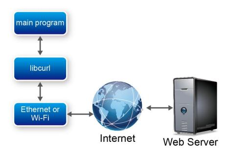
Figure 6-10 Function block diagram of Internet Time demonstration
