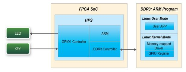
Figure 6-1 Block diagram of GPIO demonstration
