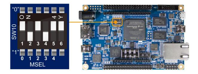
Figure 3-1 DIP switch (SW10) setting of FPPx32 mode.
