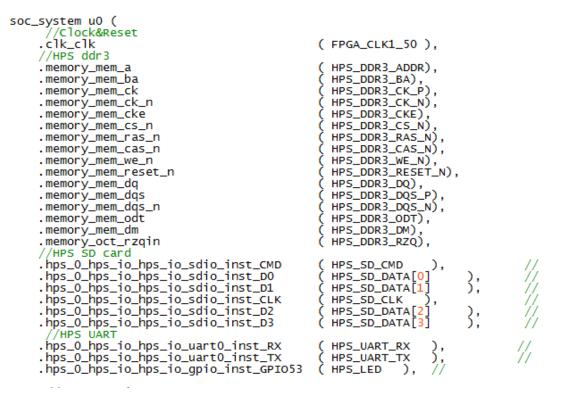
Figure 5-11 Pin connections on Quartus top
