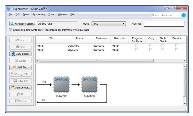
Figure 3-7 FPGA and HPS detected in Quartus programmer
