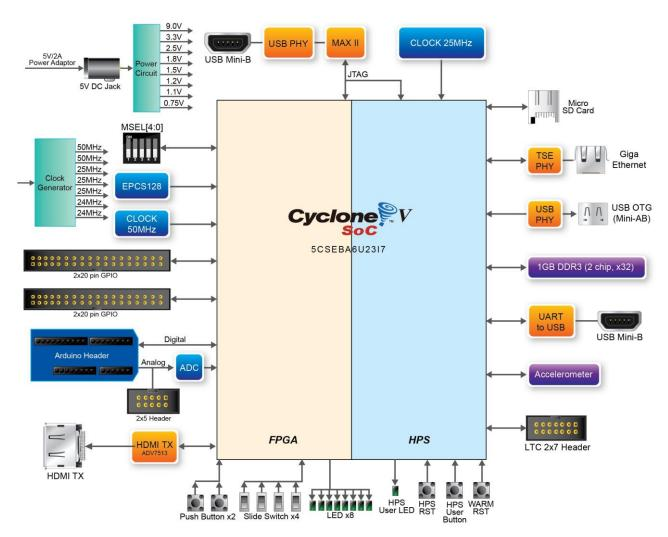
Figure 2-3 Block diagram of DE10-Nano
