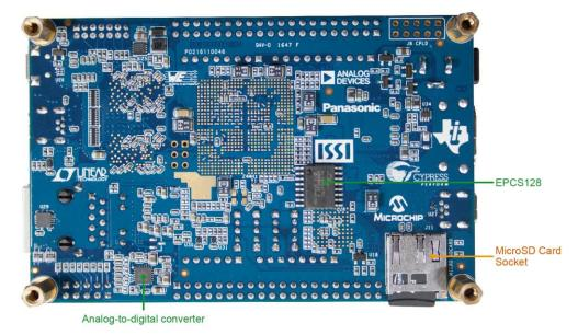
Figure 2-2 DE10-Nano development board (bottom view)
