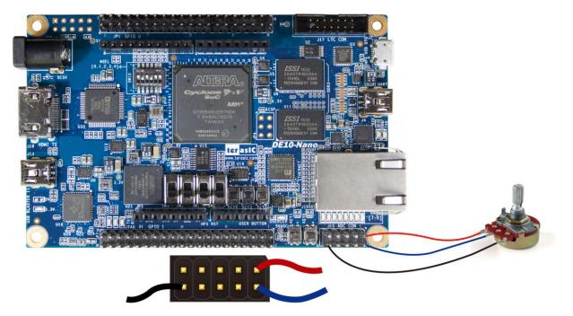
Figure 5-4 Hardware setup for the ADC reading demonstration
