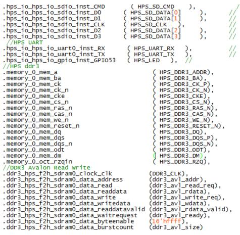
Figure 5-16 Pin connections on Quartus top
