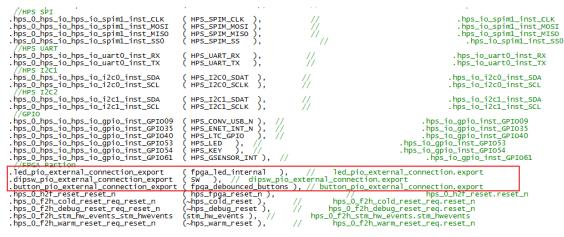
**Figure 7-3** Connection in the top design
