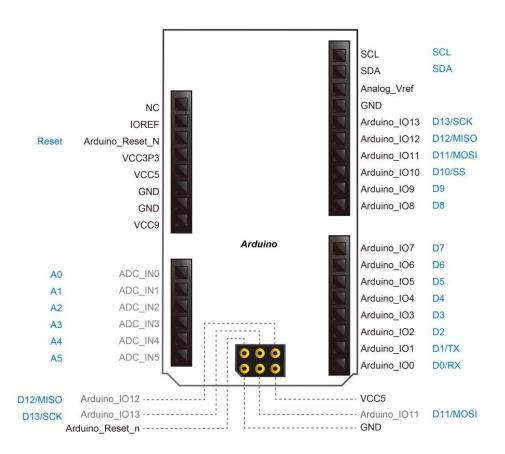
Figure 3-21 lists the all the pin-out signal name of the Arduino Uno connector. The blue font represents the Arduino pin-out definition.
