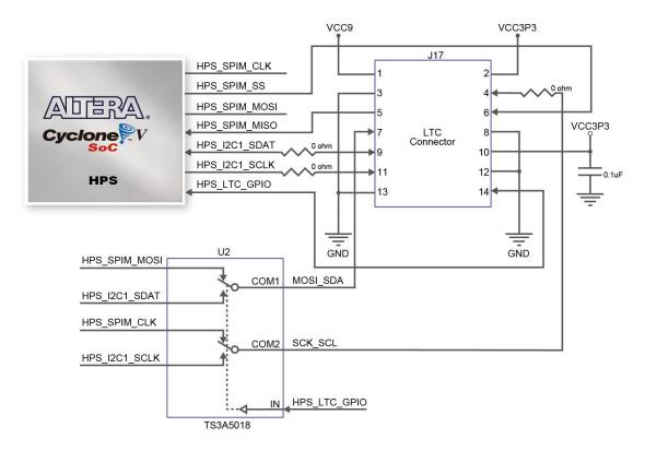
Figure 3-30 Connections between the HPS and LTC connector
