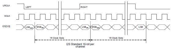
Figure 5-6 I2S standard audio with 16-bit per channel
