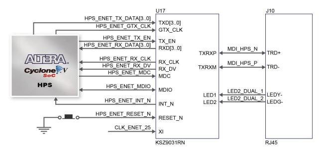
Figure 3-23 Connections between the HPS and Gigabit Ethernet
