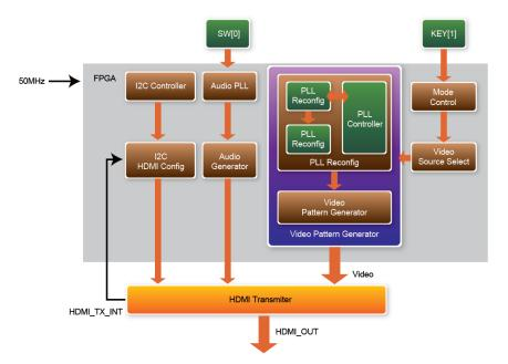
Figure 5-5 Block Diagram of the HDMI TX Demonstration
