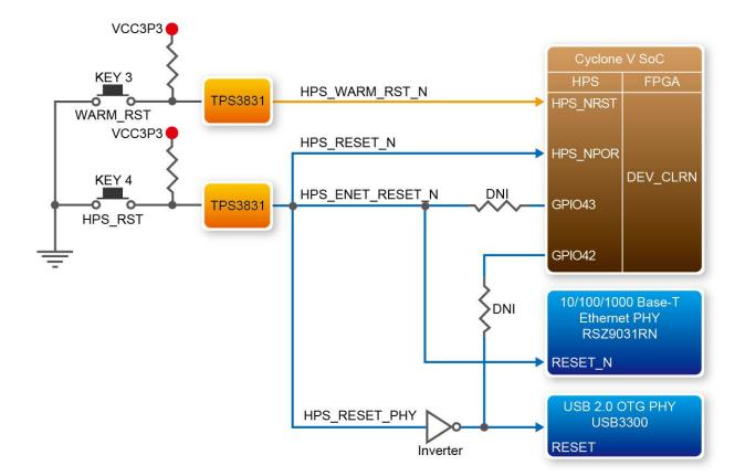
Figure 3-14 HPS reset tree on DE10-Nano board
