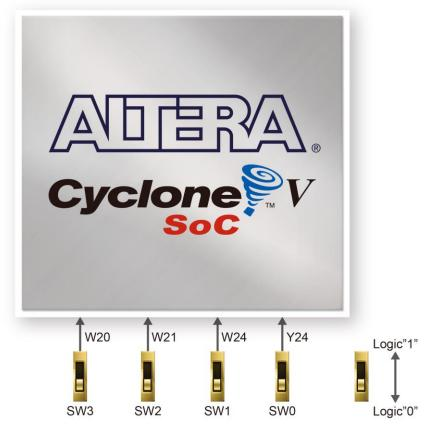
Figure 3-18 Connections between the slide switches and the Cyclone V SoC FPGA
