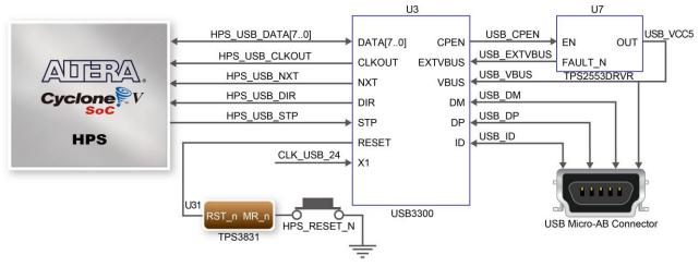
Figure 3-28 Connections between the HPS and USB OTG PHY
