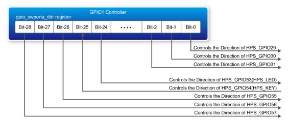
Figure 6-5 gpio\_swporta\_ddr register in the GPIO1 controller
