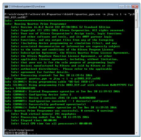
Figure 5-12 Launch the DDR3\_VIP demonstration from the ''demo\_batch'' folder
