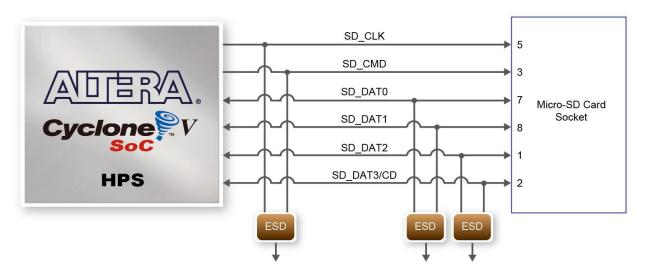
Figure 3-27 Connections between the FPGA and SD card socket
