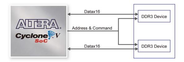
Figure 3-26 Connections between FPGA and DDR3
