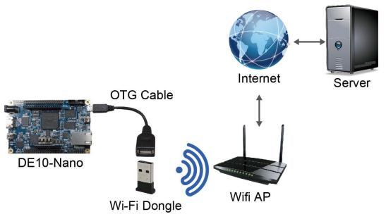
Figure 6-9 System diagram of USB Wi-Fi dongle
