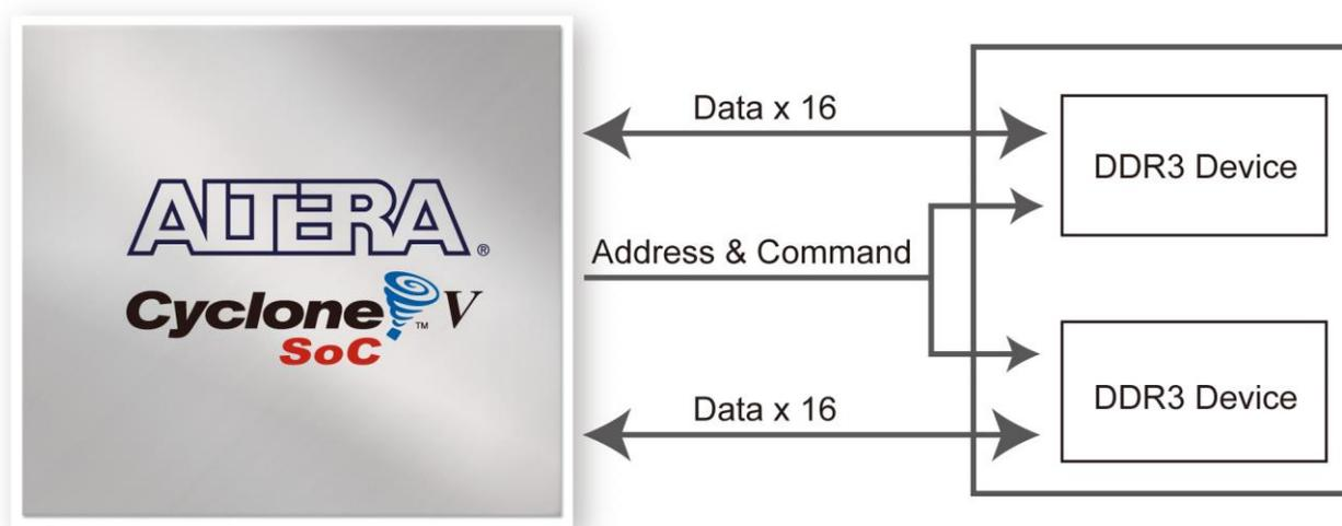
Figure 3-35 Connections between FPGA and DDR3
