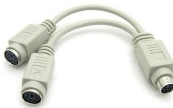
**Figure 3-30 Y-Cable for using keyboard and mouse simultaneously**
