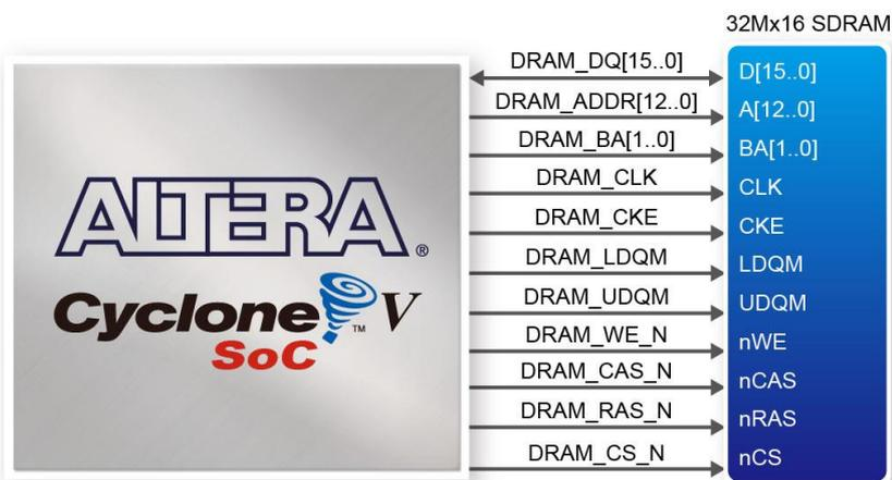
Figure 3-28 Connections between the FPGA and SDRAM
