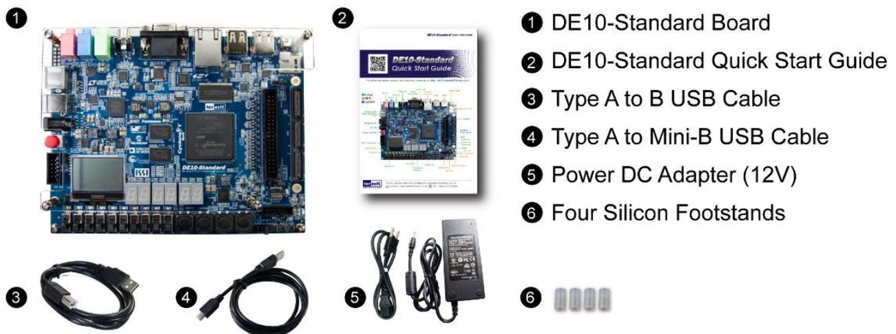
Figure 1-1 The DE10-Standard package contents
