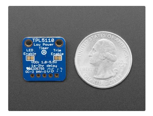
Comes as a fully assembled breakout board with a TPL5110 chip, all components onboard, and some header. A little light soldering is required to put it together for breadboard use.
