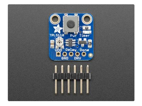
Usage is easy. First, disconnect from power and set your desired delay by adjusting the on-board trim pot: all the way to the left is once-per-100ms an all the way to the right is once-every-2-hours. Then, connect VDD up to your 3-5V power supply and then your project's power-in to the Drive pin. Finally, select a signal pin from your project to the Done pin. In your project's code or design, just make sure that it sets the Done pin high once it is completed with its task. That's it!
