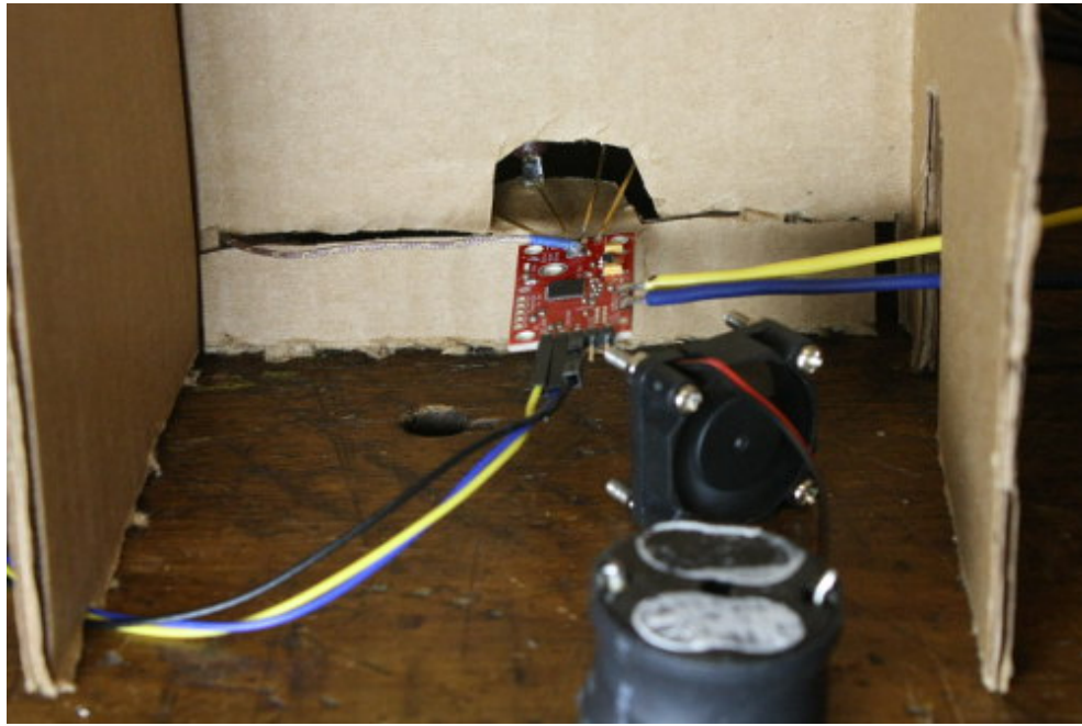
Illustration 7: Forced air cooled test
