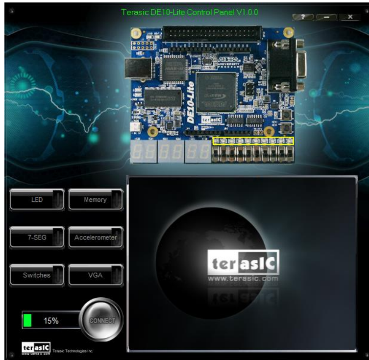
Figure 2-1 The DE10-Lite Control Panel
