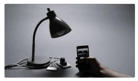
A Feather board without ambition is a Feather board without FeatherWings! This is the Power Relay FeatherWing. It gives you power to control, and control over power. Put simply, you can now turn on and off lamps, fans, solenoids, and other small appliances that run on up to 250VAC or DC power using any Feather board. <u>Compar</u> <u>ed to our smaller mini Relay FeatherWings</u> (https://adafru.it/xDL), this one can handle a beefy 1200 Watts!
