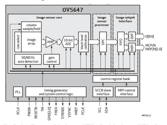
Note: Raspberry Pi camera module only support MIPI interface, it doesn't support DVP interface.
