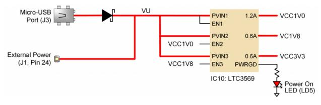
Figure 1.1. Cmod A7 Power Supply.
