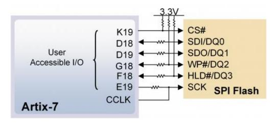
Figure 4.1. Cmod A7 Quad-SPI Flash.
