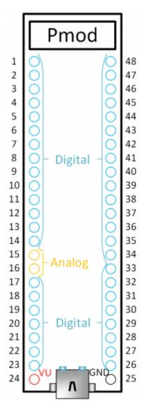
Figure 7.1. DIP pin diagram.
